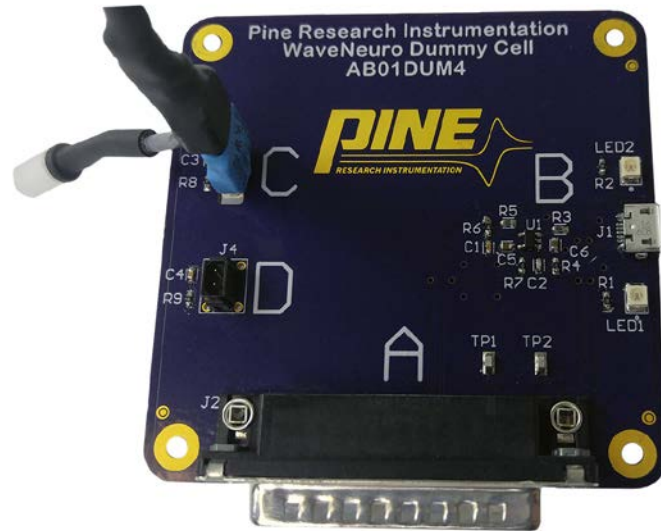
Figure 5-10. Connection of Headstage Cable to Dummy Cell C Connector
