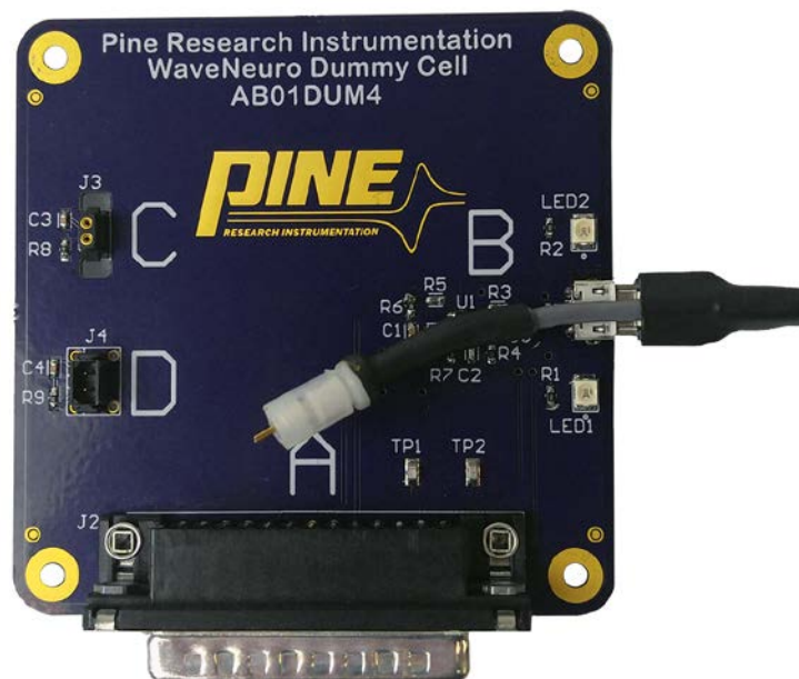
Figure 5-9. Connection of Headstage Cable to Dummy Cell B Connector
