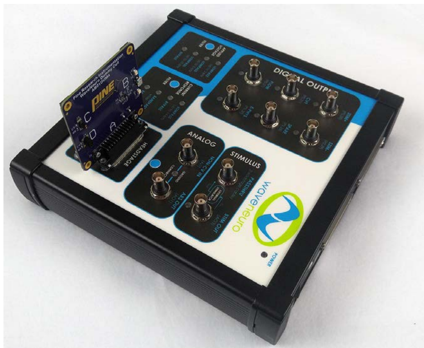
Figure 5-7: Connection of Dummy Cell to WaveNeuro HEADSTAGE Connector
