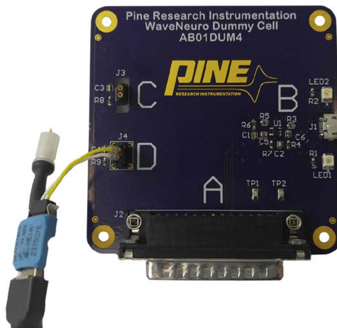
Figure 5-11: Connection of Headstage Cable to Dummy Cell D Connector.
