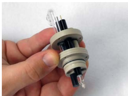
Figure 2-5. Attachment of the Lower Cap onto Thin Cap/Electrode Assembly.
