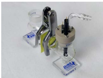
Figure 2-7. Install Cap into LowVolume Cell.
