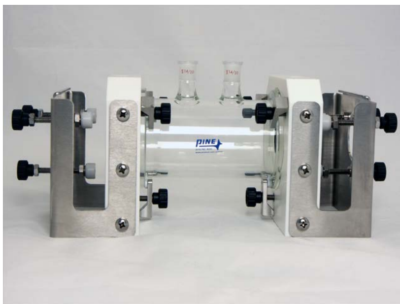
Figure 16. Proteus Alpha Cell End Assemblies Connected to Glass Cell Body
