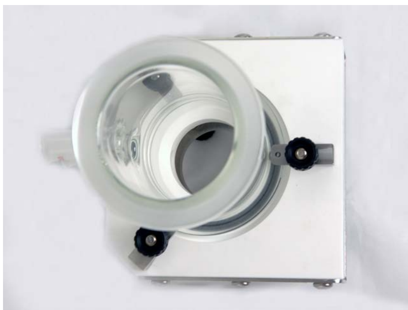
Figure 14. Attachment of the Cell Body to the First End Assembly (Vertically Oriented)
