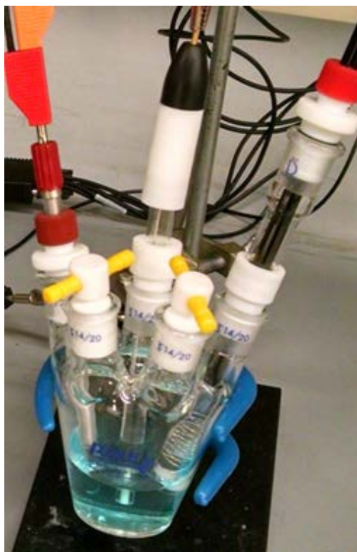
Figure 5. Standard Voltammetry Cell with PTFE Stoppers
