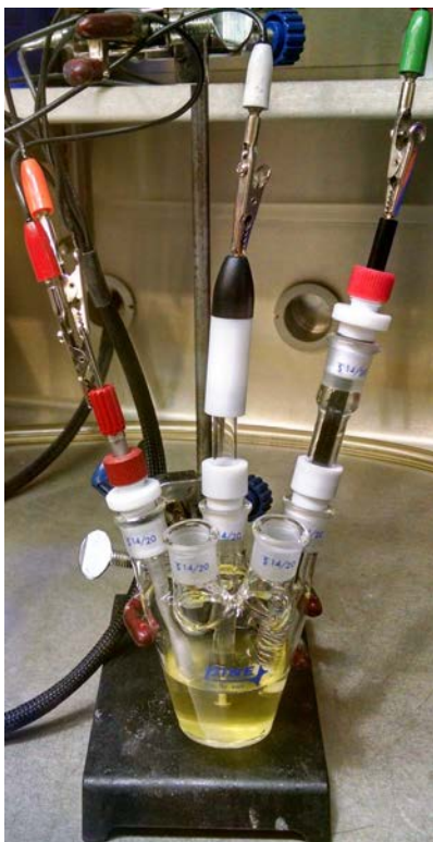
Figure 11. Electrochemical Cell Setup in the Glovebox
