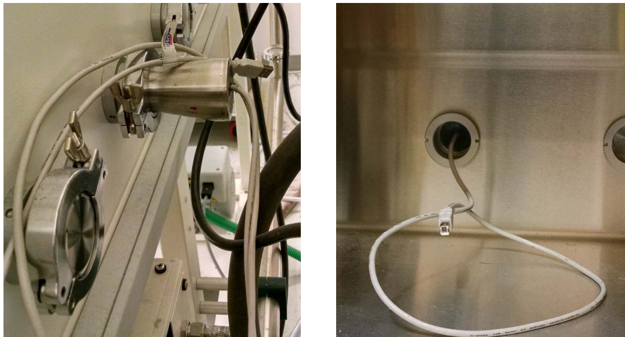
Figure 9. Commercially Installed USB Cable Feedthrough Based on KF Flange
