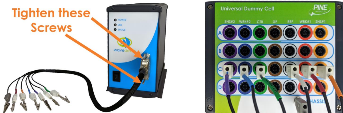
Figure 9-2. WaveDriver 40 Cell Cable Connected to Universal Dummy Cell Row “C”
