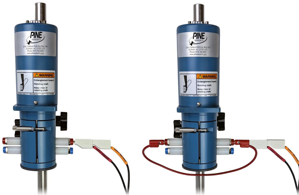
Figure 5-7. Working Electrode Connection for a Rotating Disk or Rotating Cylinder Electrode
