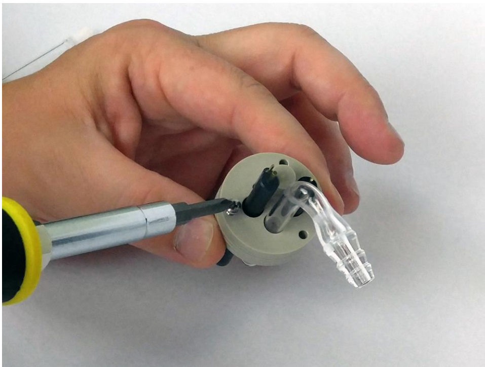
Figure 1-8. Install a screw to join the two cap halves. Loosely tighten one screw at a time to appropriately balance the cap seal.
