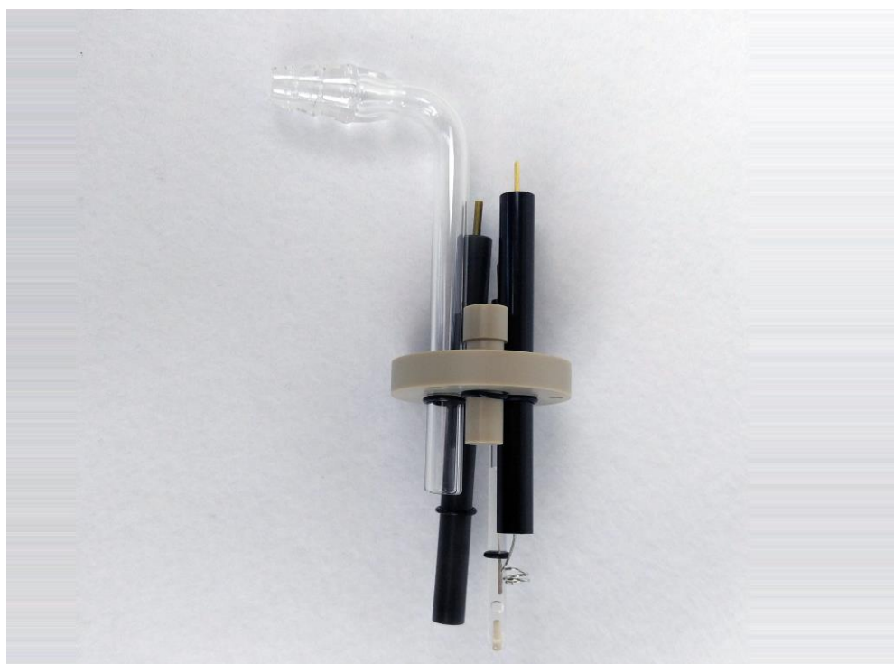
Figure 1-10. Repeat the probe and O-ring insertion for each type of electrode, plug, or glass tube. Take special caution to appropriately adjust the height of the O-ring to ensure the assembled cap will fit into the cell without the probes hitting the bottom of the cell surface.
