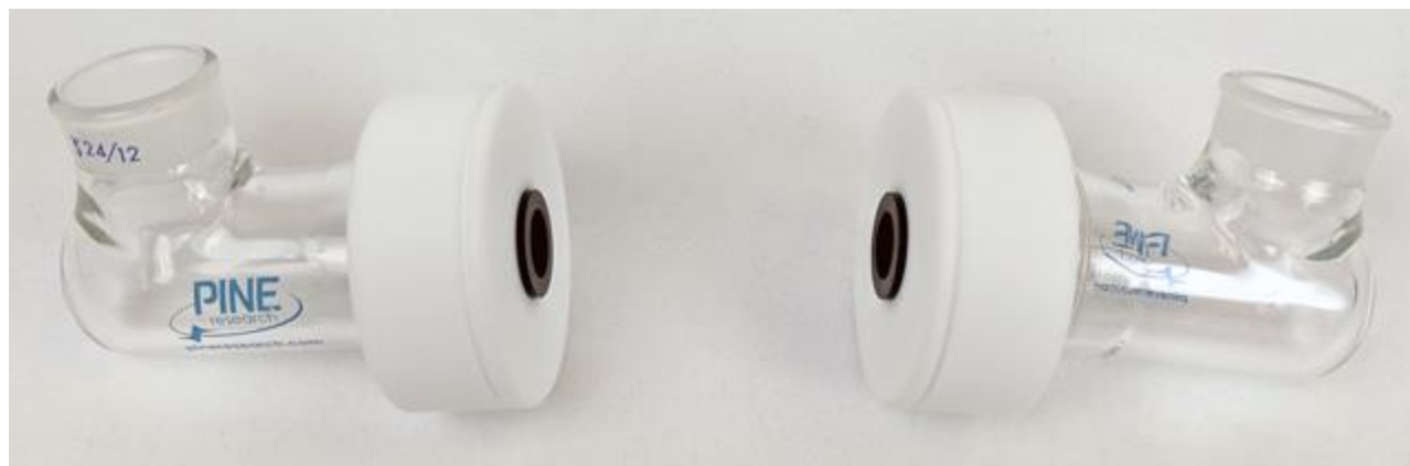
Figure 1-5. Glass half cells inserted into PTFE pucks
