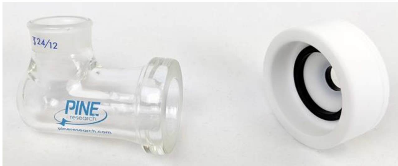
Figure 1-4. Glass half cell with PTFE puck and both O-rings installed
