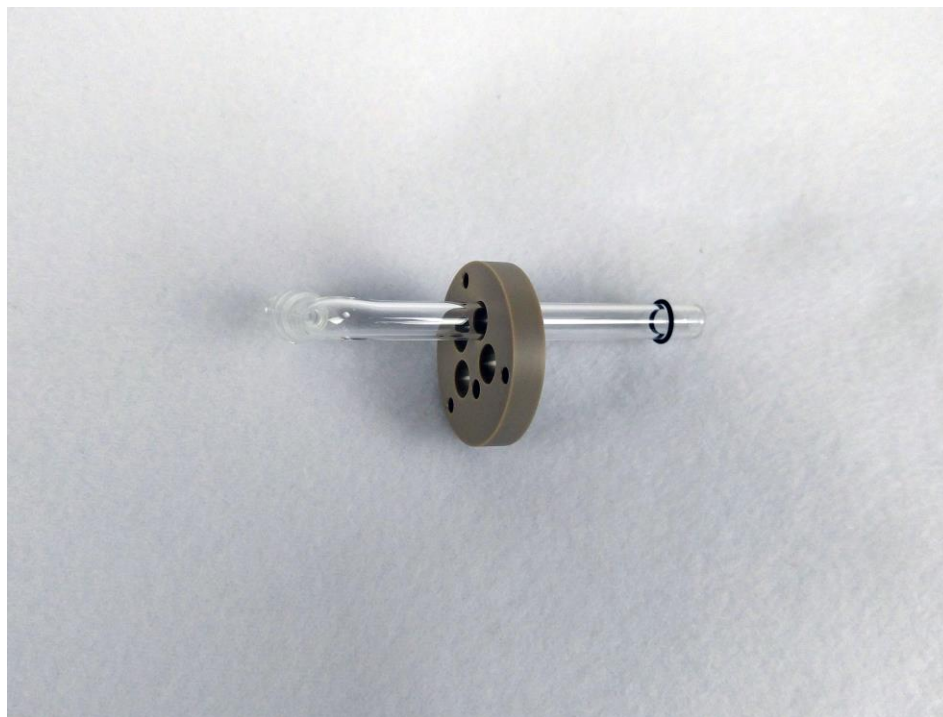
Figure 1-9. With the thin aspect of the cap kit, insert a probe (a purge tube in this image) through the appropriate hole and add an O-ring.
