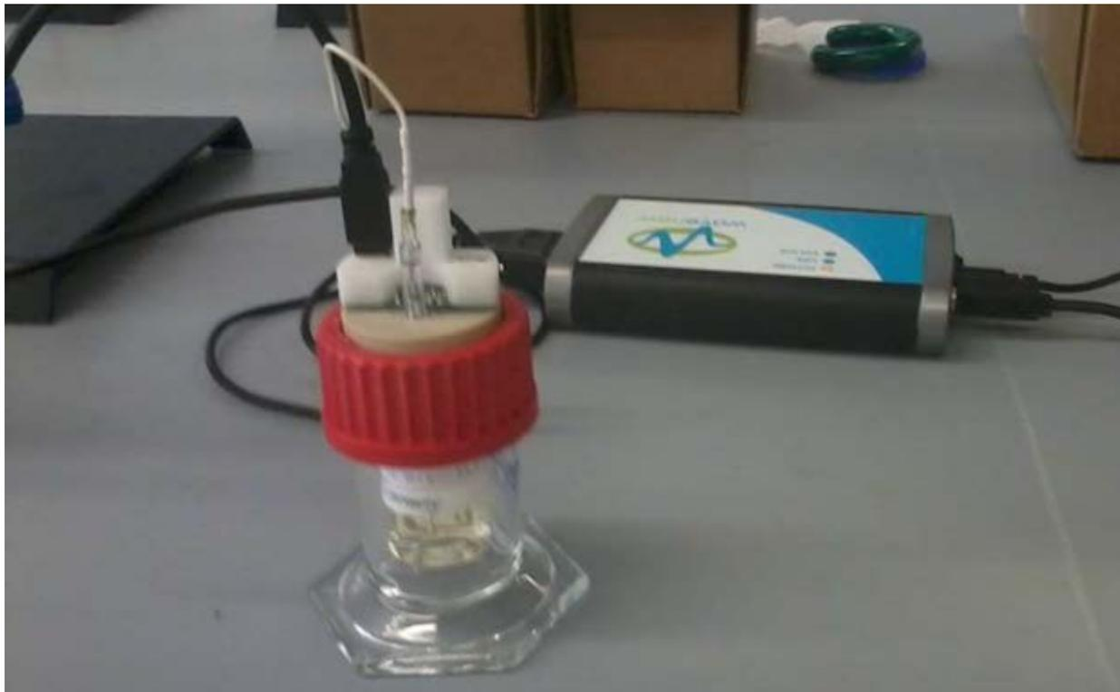
Figure 8. Mini Electrochemical Cell Setup
