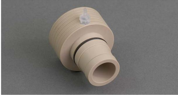
The bearing assembly should be installed onto the shaft before the shaft is installed into the MSR rotor. Slide the tapered end of the bearing assembly over the 1/4" stainless steel end of the 15 mm RCE shaft. Continue sliding the bearing assembly down onto the PEEK shroud of the shaft (see figure below). A retaining ring on the shaft will keep the bearing assembly in place during its installation into the MSR Rotor.
