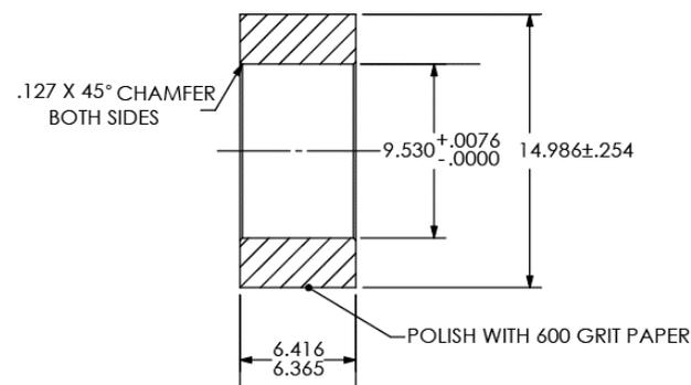
Cylinder inserts are sold in packages of ten (10). Each package includes a certification sheet for the material used to manufacture the cylinder inserts. The cylinder inserts made by Pine Research are fabricated from a variety of popular steel alloys.
