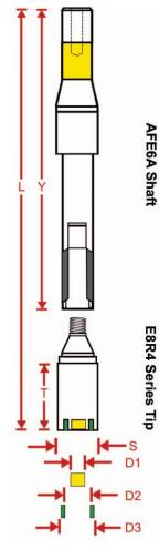
Disk Diameter (D1): 5.0 mm6.0 mm Ring ID (D2): 8.5 mm Ring OD (D3): Shroud Diameter (S): 15.0 mm Tip Shroud Length (T): 25.4 mm Overall Length (L): 184.2 mm Shaft Length (Y):  $158.0 \ mm$ **Collection Efficiency:** 43.9%
