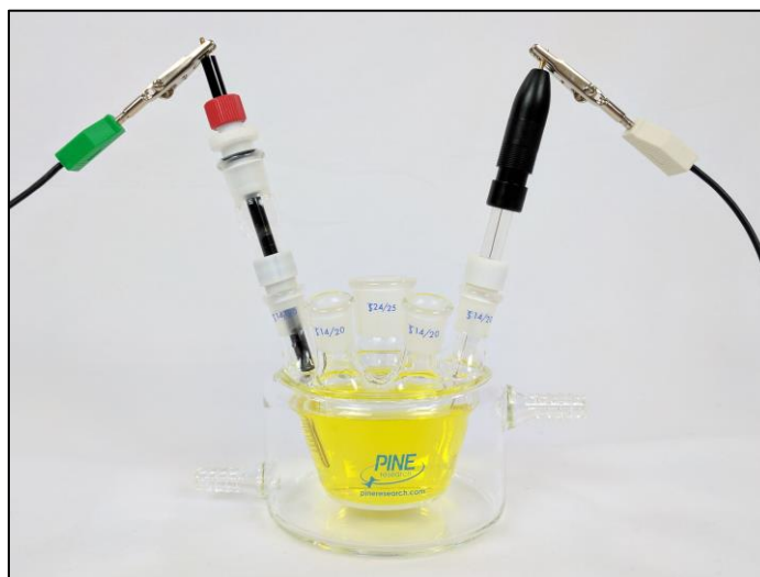
Figure 4.7: Connection of Counter and Reference Electrodes
