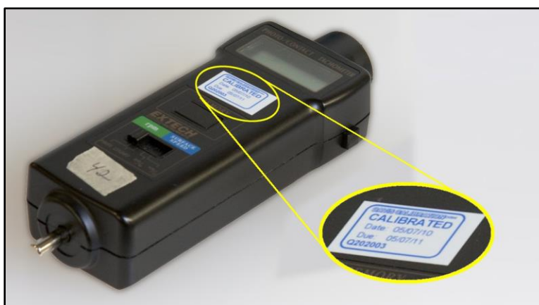
Figure 6.2: Professional Optical Tachometer with Traceable Calibration
