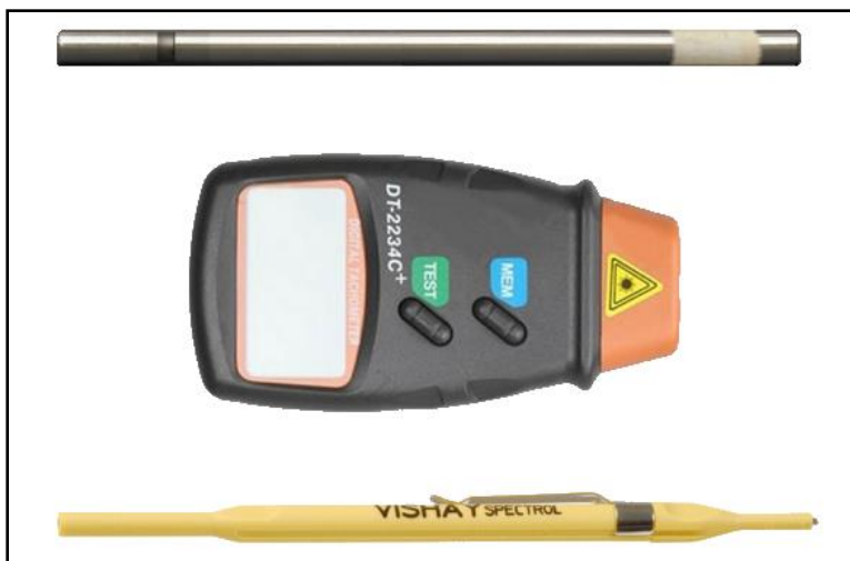
Figure 6.1: Rotator Calibration Toolkit (including simple handheld tachometer)
