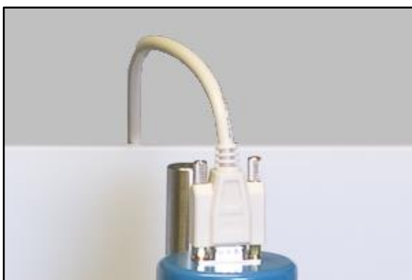
Figure 4.11: Routing Cables out of the Enclosure
