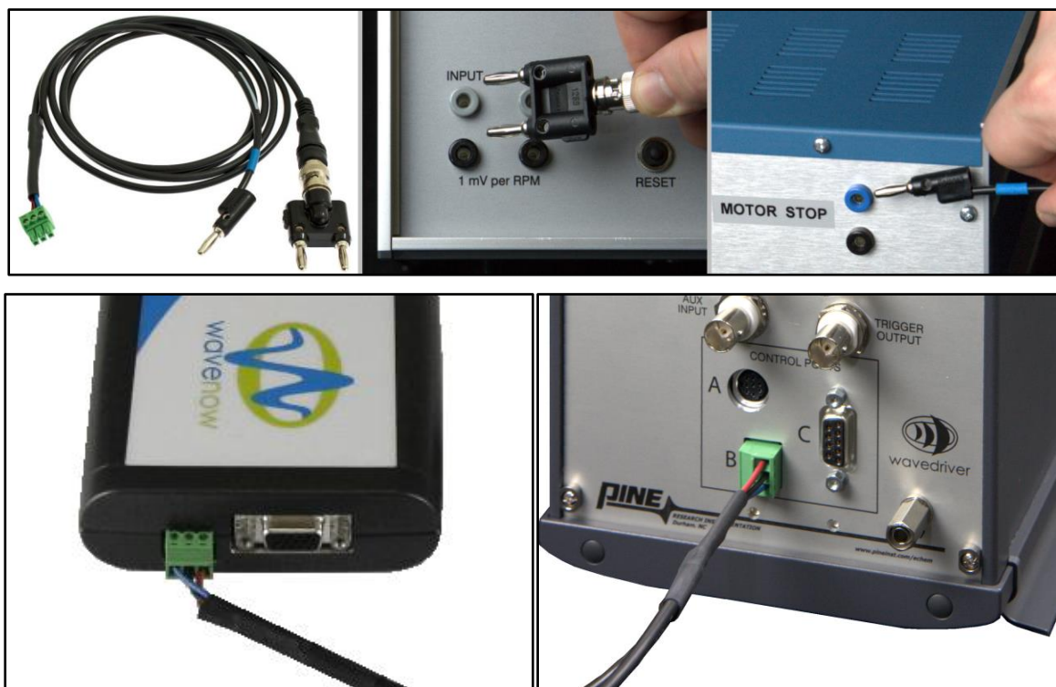
Figure 4.15: Connecting the Rotation Rate Control Cable
