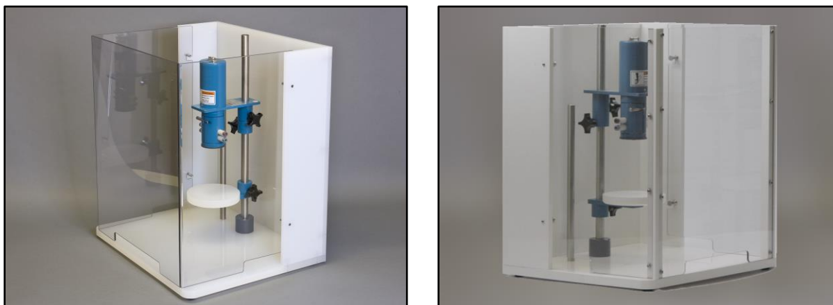
Figure 2.2: Two Styles of Enclosure Window
