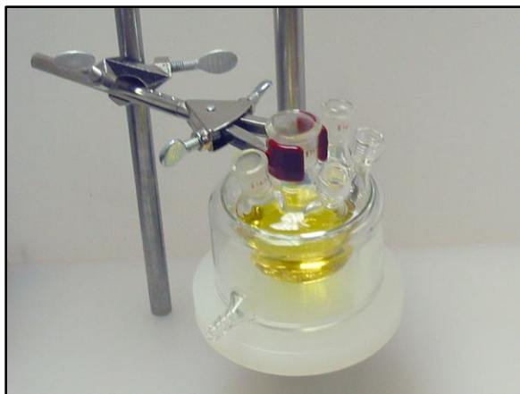
Figure 4.5: Properly Supported and Clamped Electrochemical Cells
