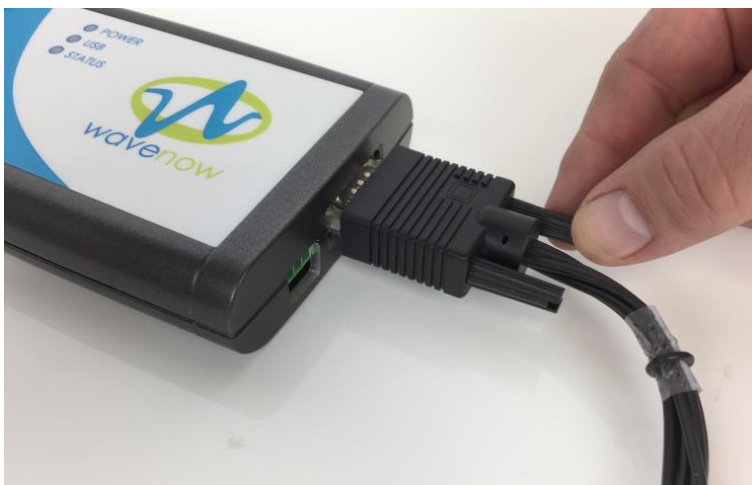
Figure 5-2. Securely Tighten the HD-15 Connector to the Cell Port
