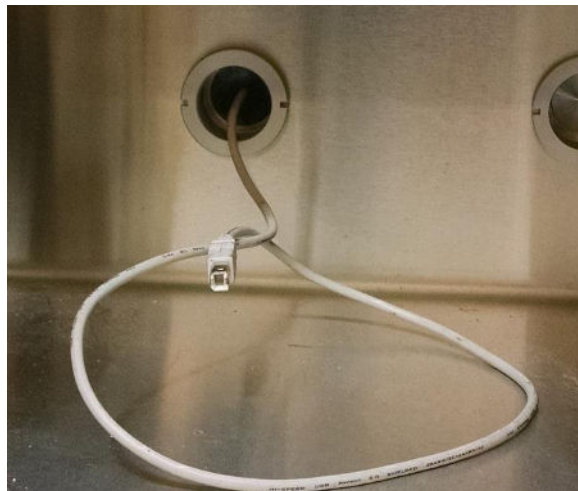
Figure 3-1. USB Cable Glovebox Feedthrough
