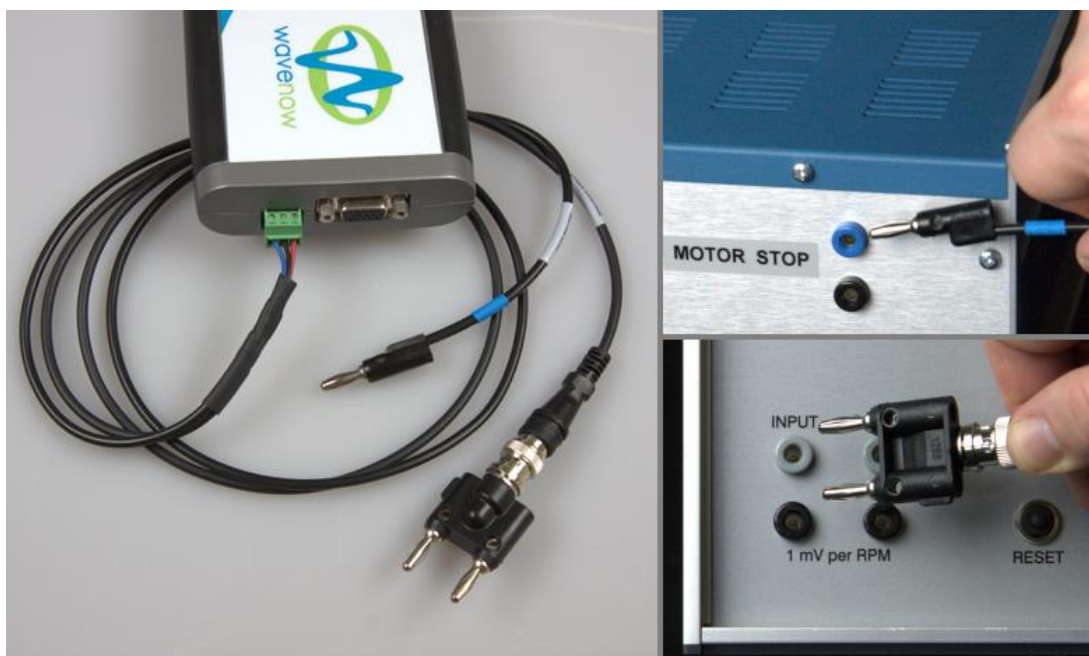
Figure 5-7. Rotation Rate Control Connections for a Pine Research MSR Rotator
