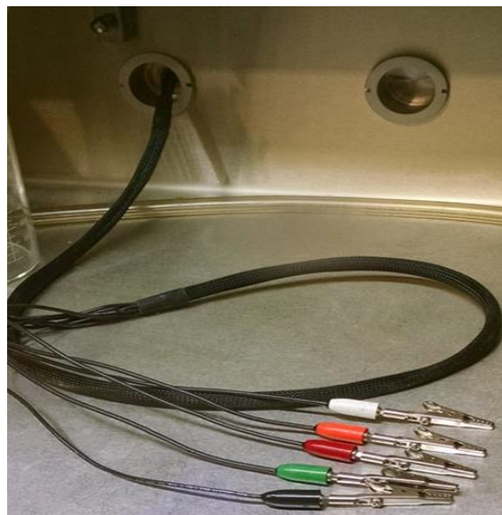
Figure 3-2. Cell Cable Glovebox Feedthrough
