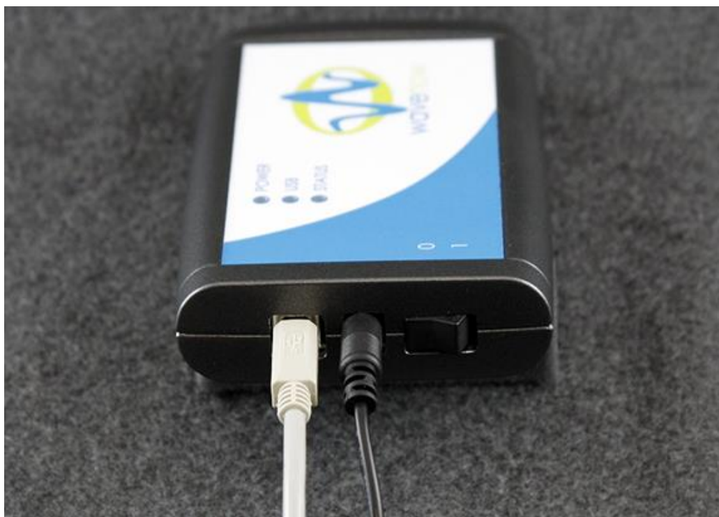
Figure 3-5. USB Cable Connection between Potentiostat and Computer
