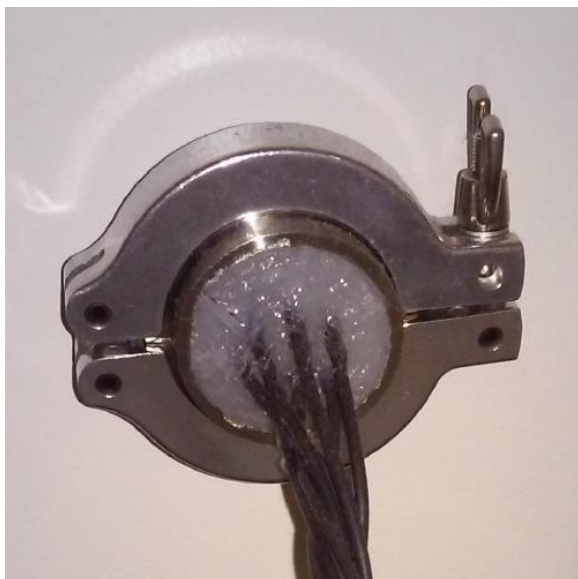
Figure 3-2. Cell Cable Glovebox Feedthrough
