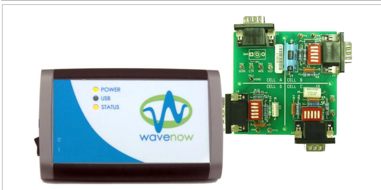
Figure 2-5. Dummy Cell Connected to the WaveNow
