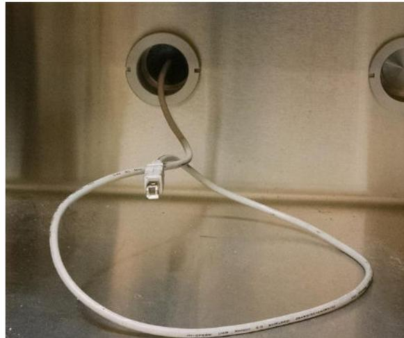
**Figure 3-1. USB Cable Glovebox Feedthrough**
