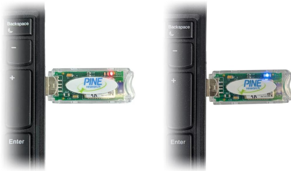
Figure 3-19. Wireless USB Dongle Indicating Connection Status (Red or Blue)
