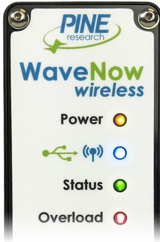
Figure 3-20. Instrument Light Status during Wireless Connection (Blue)
