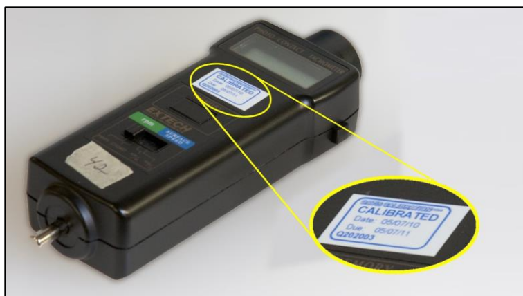
Figure 6-2. Professional Optical Tachometer with Traceable Calibration
