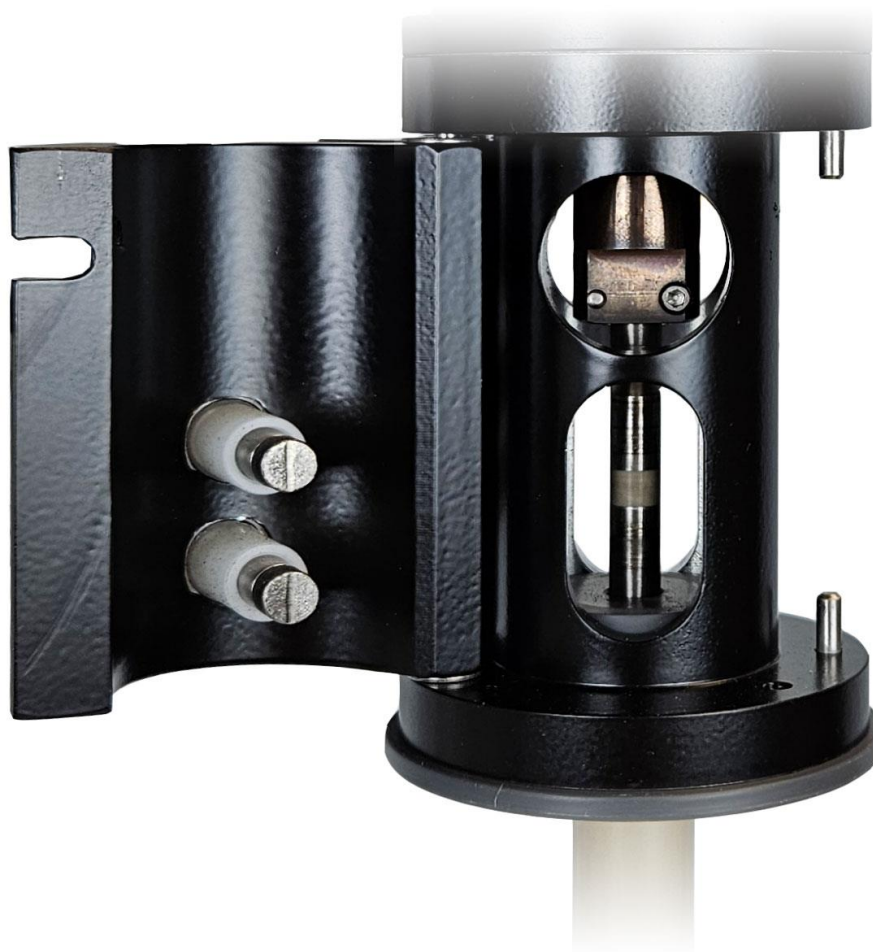
Figure 4-2. MSR evo Brush Chamber (Side View)
