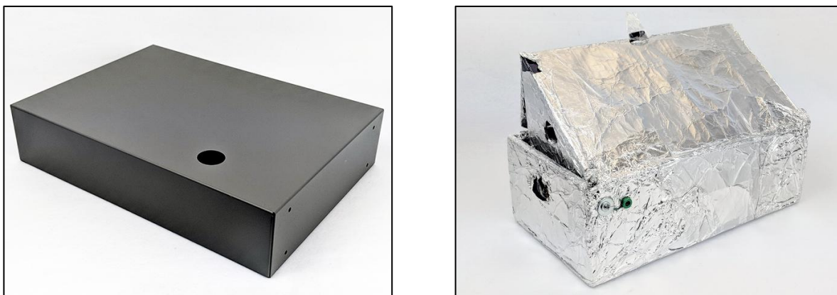
Figure 4-16. Common Examples of Faraday Cages
