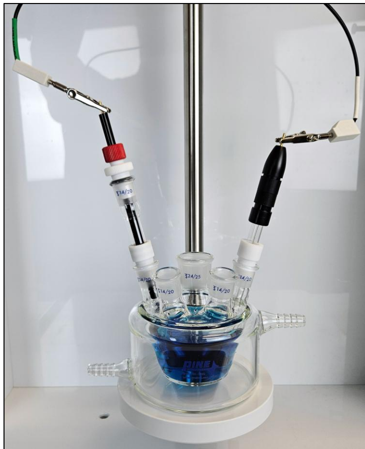
Figure 4-7. Connection of Counter and Reference Electrodes
