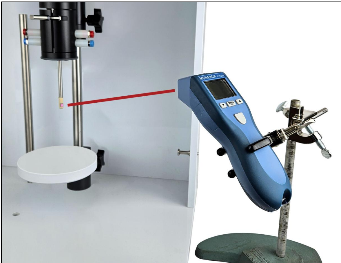
Figure 6-2. Use of Optical Tachometer with Reflective Target
