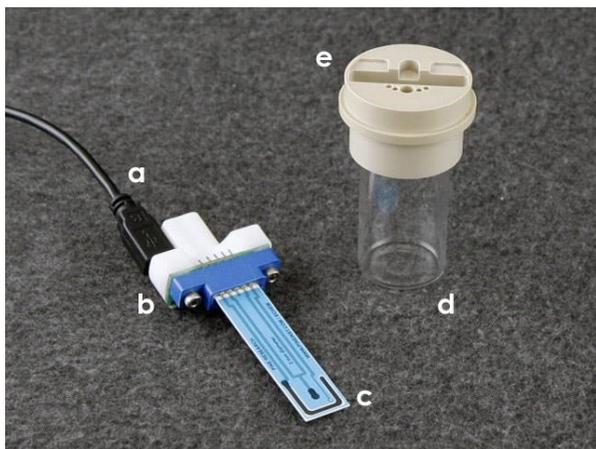
Figure 5. Compact Voltammetry Cell Components
