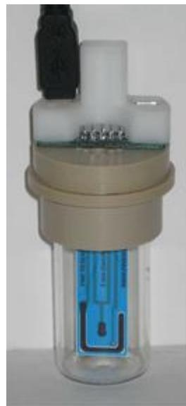
Figure 6. Assembled Compact Voltammetry Cell, USB Cable Connected to the Left
