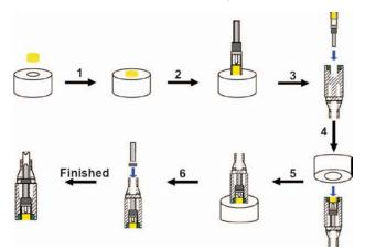
Set the mounting block on a flat surface with the small bore facing upwards. Carefully drop the disk insert into the mounting block. The polished surface of the disk insert should face downwards. The disk insert should be centered and should rest in a shallow well located within the small bore.
