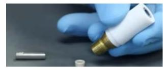
Fully loosen the screw on the disk core ejector. Mount the disk core ejector by threading the big cylinder over the matching male threading on the electrode tip. Advance the big cylinder forward until stopped by the tip. Turn the disk core ejector screw slowly until the disk core assembly is completely pushed out of the tip body. Remove the disk assembly carefully, making sure not to scratch the disk. The disk can now be safely removed from the assembly.
