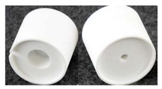
Care should be taken when handling the disk insert so that the front (polished) side of the disk is not scratched or damaged. Wear disposable gloves when working with the disk insert (to avoid contamination of the disk insert with skin oils). To use the mounting bock to install the disk insert in the disk holder, use the illustration and steps listed below.
