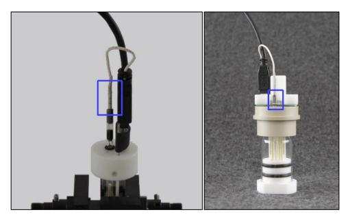
Figure 5-11. Compact Voltammetry and Spectroelectrochemical Cells with Separate Reference Electrode Connections
