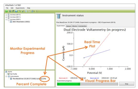
Figure 4-12. Monitoring the Progress of the Dual Channel Test (K1 and K2)
