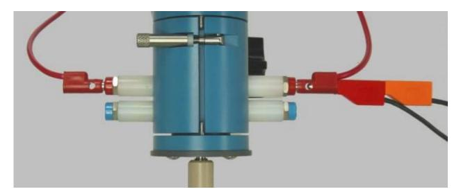
Figure 5-7. Working Electrode Connections for Rotating Disk or Cylinder Electrodes
