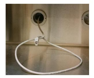
Figure 3-1. USB Cable Glovebox Feedthrough
