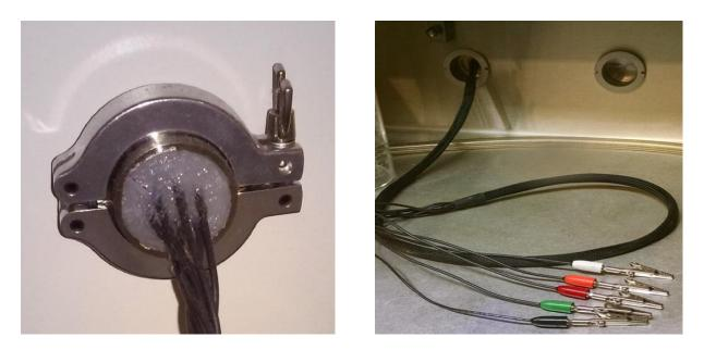
Figure 3-2. Cell Cable Glovebox Feedthrough
