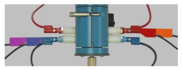
Figure 5-8. Electrode Connections (K1 and K2) for a Rotating Ring-Disk Electrode
