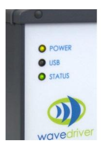
Figure 4-3. LED Status Light on the Front Panel of the WaveDriver 10 or WaveDriver 20
