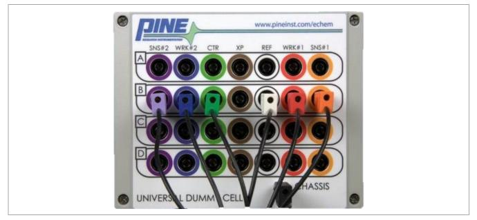
Figure 2-6. Universal Dummy Cell Connected to the WaveDriver 20
