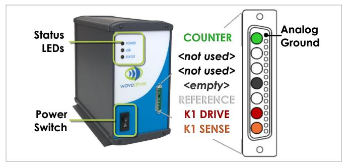
Figure 2-1. Front Panel of the WaveDriver 10
