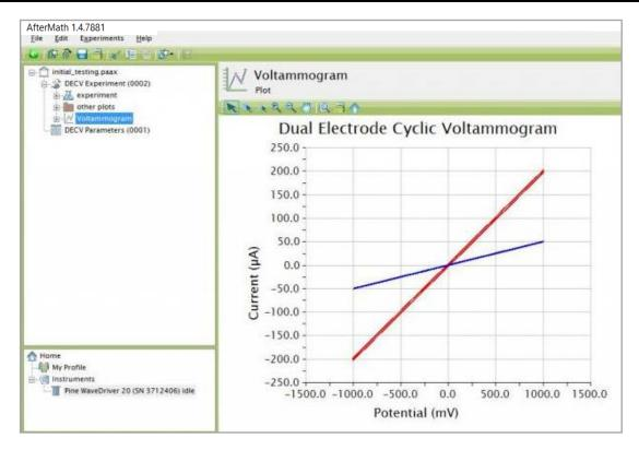
Figure 4-13. Anticipated DECV Results (using Dummy Cell B)
