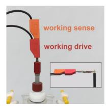
Figure 5-6. Connect Working Electrode Sense and Drive Lines Together Near the Cell
