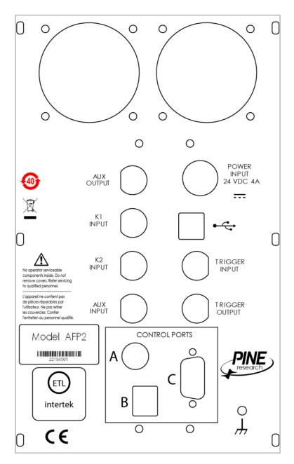
Figure 1-1. WaveDriver Back Panel Markings
