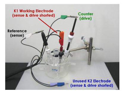
Figure 5-5. Traditional Three-Electrode Cell Connections
