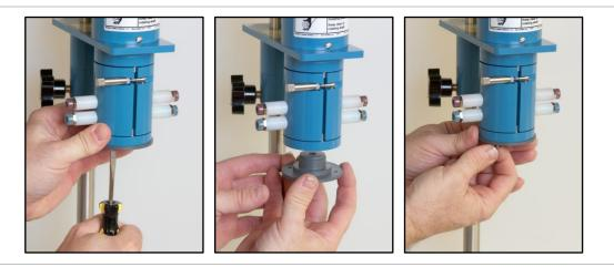
Disconnect the motor control cable from the connector on top of the motor unit. If there is a shaft presently installed the motor unit, remove the shaft. Disconnect any signal cables from the brush banana jacks (red and blue).
