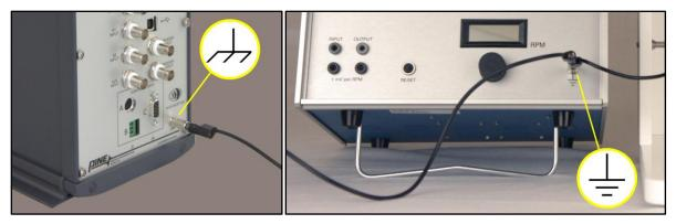
Figure 4.13: Connect Potentiostat to Earth Ground on Control Box Front Panel
