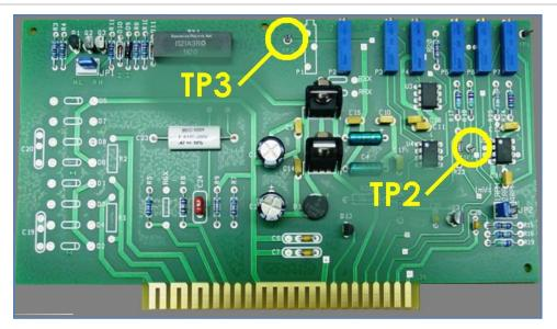
Locate testpoints **TP2** and **TP3** on the circuit board. These testpoints are accessible without the need to remove the circuit board from the control unit.
