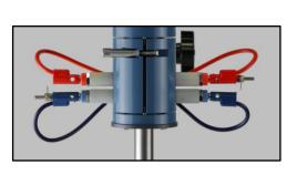
two short There are banana cables (red and blue) which serve as jumpers between the left and riaht brush connections. Use the red cable to connect the upper (red) pair of brush connections, and use the blue cable to connect the lower (blue) pair of brush connections, running the wires behind the assembly as shown.
