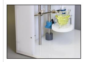
There are several holes in the floor of the enclosure base (4), which are threaded to accept the side post (6). Choose one of these holes and install the side post in it. Then, mount the laboratory clamp on to the side post.
