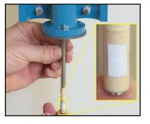
While the power is switched off, install the tachometer target into the motor coupling on the motor unit.
