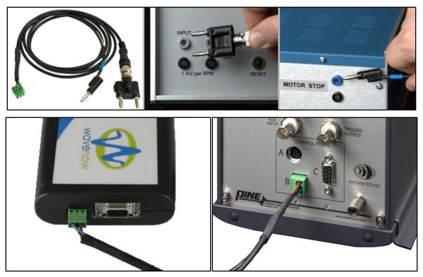
Figure 4.15: Connecting the Rotation Rate Control Cable
