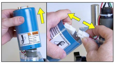
The internal cables are secured to the motor using two plastic cable ties. In order to remove the motor, the lower cable tie must be cut and removed.
