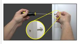
Locate the small bag of hardware. Remove the four pins and four screws. Place each screw in one of the pre-drilled holes along the side walls of the enclosure, two on the left and two on the right. Install the pins onto the screws. Properly installed pins will point inwards as shown.
