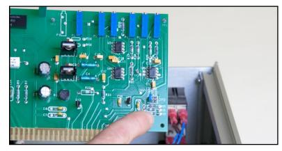
Place the jumper across one of the three pairs of pins at **JP2**. Choose the ratio required for the particular potentiostat being used with the rotator.
