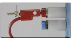
Insert one banana plug stud into the red banana cable, and insert the other banana plug stud into the blue banana cable. These flat studs are an ideal place to make connections using alligator clips.
