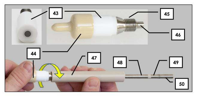
Figure 2.7: Typical Rotating Ring-Disk Electrode (RRDE) Tip with Shaft
