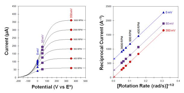
Figure 10.9: Koutecky Levich Study – Voltammograms with Sluggish Kinetics
