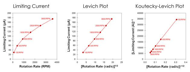
Figure 10.8: Levich Study – Limiting Current versus Rotation Rate
