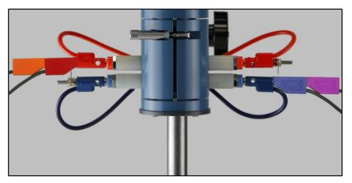
Figure 4.9: Brush Connections for a Rotating Ring-Disk Electrode (RRDE)
