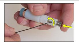
Use the small hex key to remove the set screw. Note that the required hex key (0.035") is included with the brush replacement kit.
