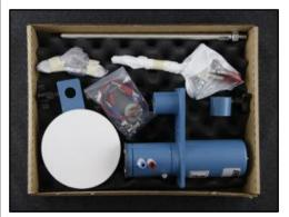
Open the smaller box. It should contain the motor unit (2), the support collar (5), the cell platform (3), the side post (6), a standard three-pronged laboratory clamp (with right-angle mount), and a small bag containing two banana cables and some additional assembly hardware.
