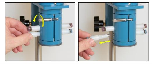
Install the new brush assembly by threading it by hand into the side of the rotator. Do not use tools to tighten the brush assembly.
