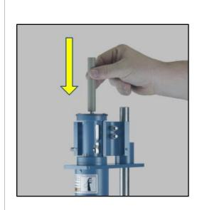
Install the shaft by sliding it through the hole in the lower bearing assembly and into the brush chamber.
