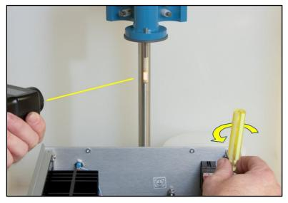
Figure 6.3: Use of Optical Tachometer with Reflective Target
