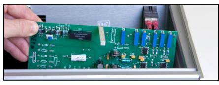
On the board, locate the configuration pins with the designation **JP2**. There is a small jumper that can be used to short together one of three pairs of pins.
