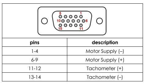
Table 6.1: Motor Control Cable Wiring
