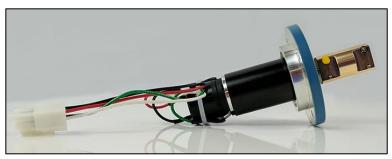
Remove any extra cable ties (i.e. around the green part of the motor) so that the cable can move freely.
