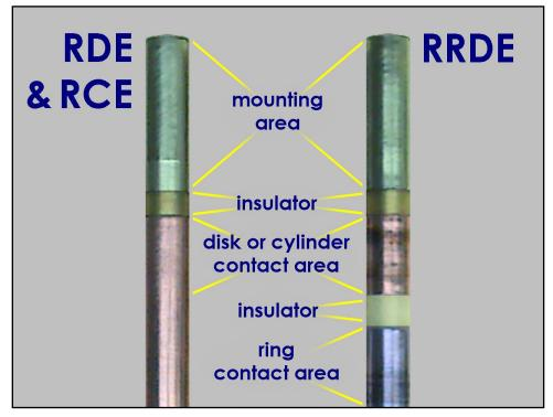
Figure 4.1: Contact Areas at Top of Rotating Electrode Shafts
