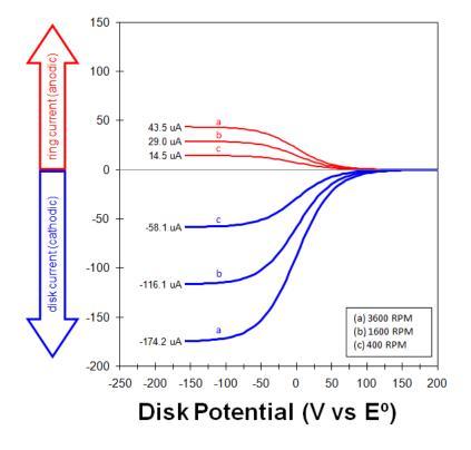
Figure 10.10: Rotating Ring-Disk Voltammograms at Various Rotation Rates
