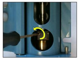
If there is a shaft already installed, use the hex driver tool (5/64", provided) to loosen the two screws on the motor coupling. Do not remove these screws entirely; just loosen them by one or two turns of the hex driver. Usually it is necessary to hold the motor coupling in place with one hand while loosening the screws with the other hand.
