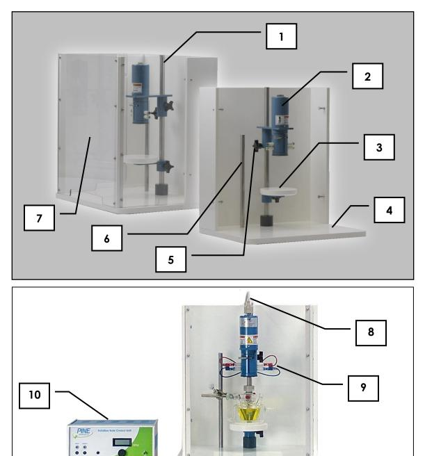
Figure 2.1: Major Components of the MSR Rotator System
