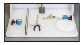
Locate the support collar (5), side post (6), and three-pronged laboratory clamp (with rightangle mount), cell platform (3), and the large plastic washer (usually shipped in the hardware bag).
