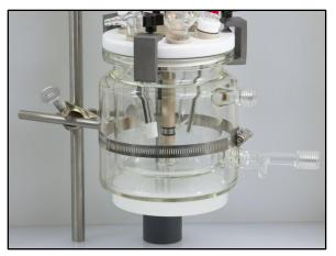
Figure 4.5: Properly Supported and Clamped Electrochemical Cells
