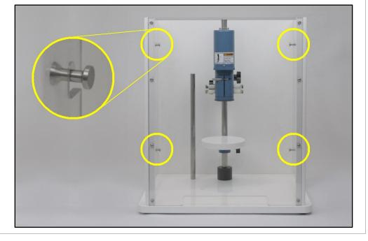
The motor unit and electrochemical cell are enclosed on the back side by a rear wall permanently attached to the enclosure base. The cell and motor are further enclosed on the front side by a transparent enclosure window. The enclosure
