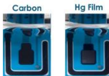
Figure 2-1. Bare Carbon Screen Printed Electrode and Mercury Plated Screen Printed Electrode
