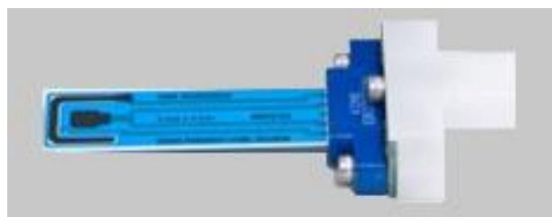
Figure 5-2. Connection between Screen Printed Electrode and Hand Grip
