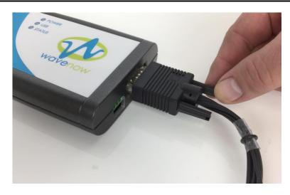
Figure 5-2. Securely Tighten the HD-15 Connector to the Cell Port
