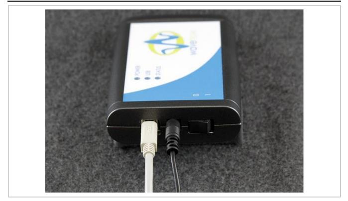
Figure 3-5. USB Cable Connection between Potentiostat and Computer
