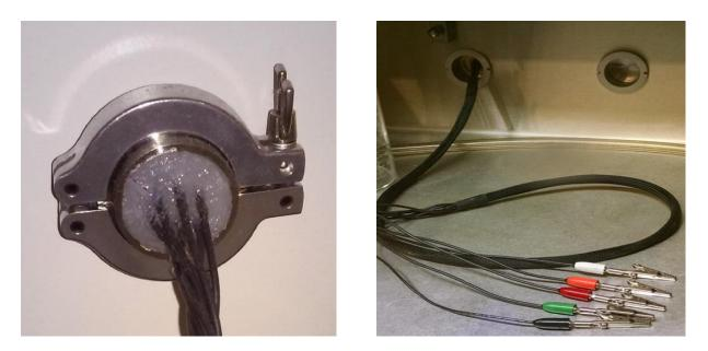
Figure 3-2. Cell Cable Glovebox Feedthrough
