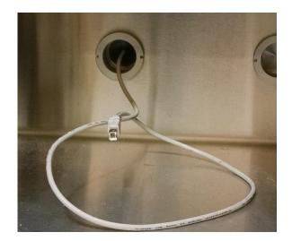
Figure 3-1. USB Cable Glovebox Feedthrough
