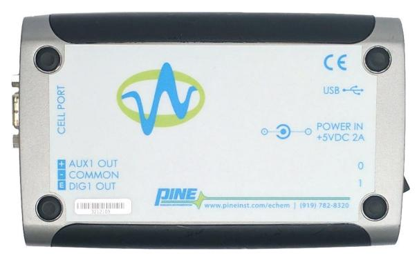
Figure 1-1. WaveNow, WaveNano, and WaveNow<sup>XV</sup> Bottom Panel Markings
