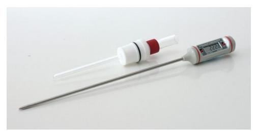
Figure 19. Digital Thermometer with Glass Well and 24/25 Port Adapter.
