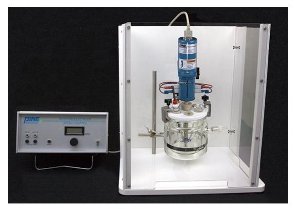
Figure 1. Typical Rotating Cylinder Setup for Corrosion Analysis.
