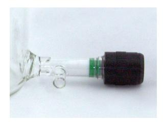
Figure 14. Threaded Drain Valve Stem with Knob.
