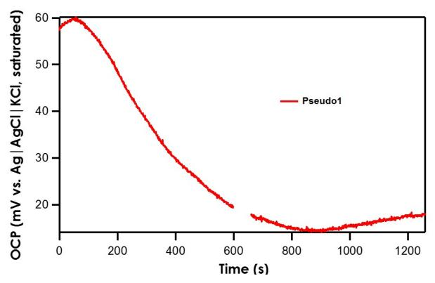
Figure 4. Relative Stability of Pseudo1 Reference Electrode with respect to the Ag|AgCl|KCl (saturated) | frit.
