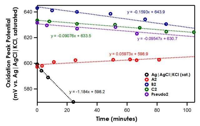
Figure 6. Oxidation Peak Position of Ferrocene with Varying Reference Electrodes in Dichloromethane.
