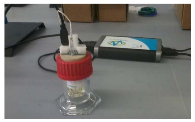
Figure 8. Mini Electrochemical Cell Setup
