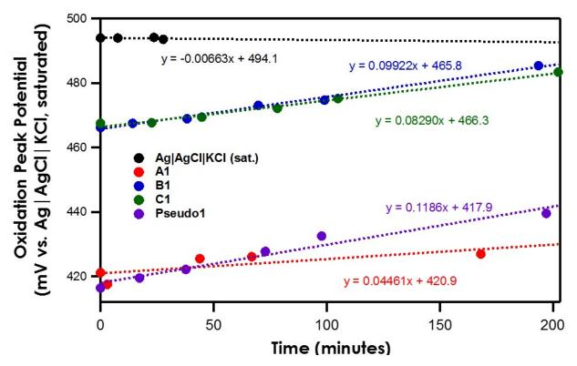
Figure 5. Oxidation Peak Position of Ferrocene with Varying Reference Electrodes in Acetonitrile.
