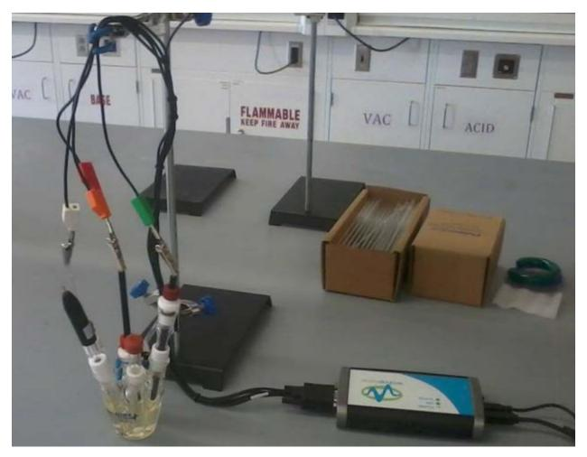
Figure 7. Electrochemical Cell (AKCELL1).
