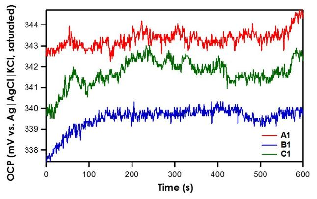
Figure 3. Relative Stability of Reference Electrodes A1, B1, and C1 with respect to the Ag|AgCl|KCl (saturated) | frit.
