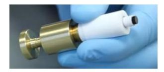
**MSR Rotator Shaft with Tip**
