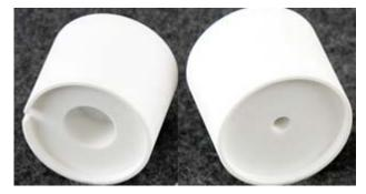
Care should be taken when handling the disk insert so that the front (polished) side of the disk is not scratched or damaged. Wear disposable gloves when working with the disk insert (to avoid contamination of the disk insert with skin oils). To use the mounting bock to install the disk insert in the disk holder, use the illustration and steps listed below.
