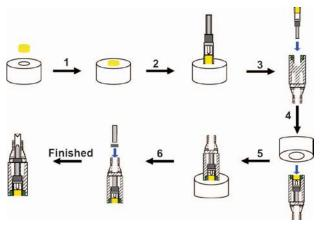
Set the mounting block on a flat surface with the small bore facing upwards. Carefully drop the disk insert into the mounting block. The polished surface of the disk insert should face downwards. The disk insert should be centered and should rest in a shallow well located within the small bore.
