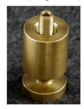
To eject the disk insert, remove the disk core nut from the electrode tip and invert the electrode tip so that the disk core washer falls out.
