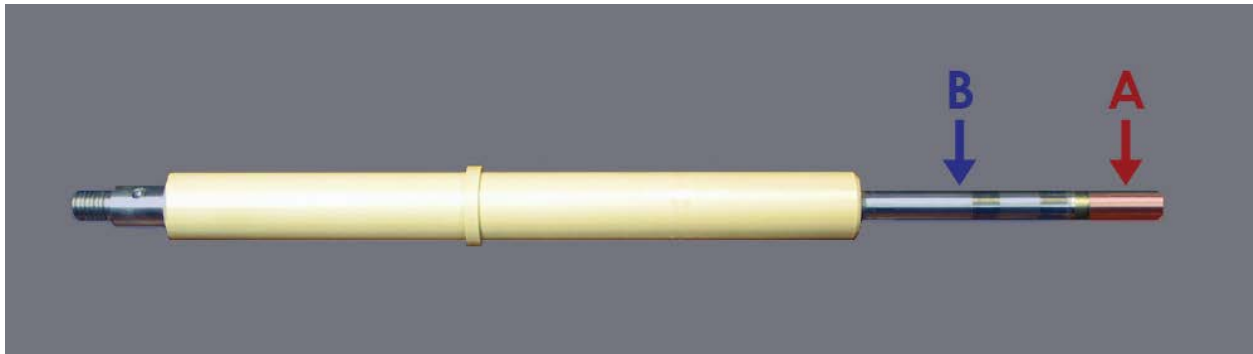
Figure 5: RCE Shaft with Electrically Isolated Sections Labeled
