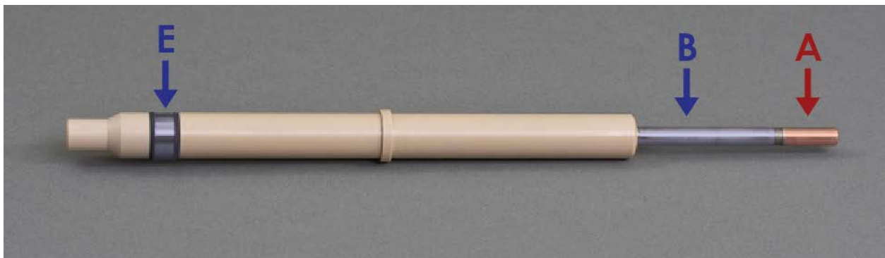
Figure 6: Electrical Isolations Labeled with Cylinder Inserted on Shaft AFE9MBA
