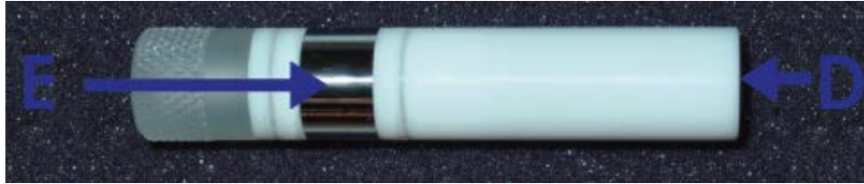
Figure 7: RCE Shaft with Electrically Isolated Sections Labeled
