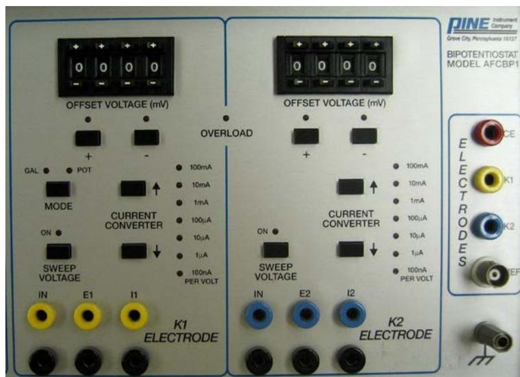
Figure 2: Front Panel (Right Side Only) of the CBP Bipotentiostat
