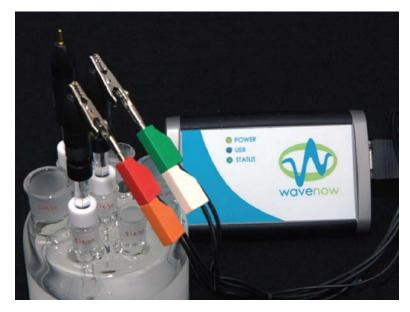
Figure 5. Reference Electrode Test with a Potentiostat
