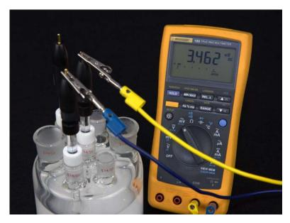
Figure 4. Reference Electrode Test with a Multimeter
