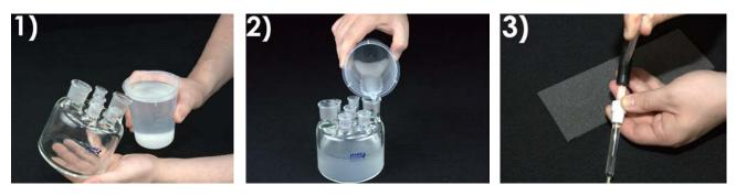
Figure 2. Steps to Construct a Master Reference Electrode
