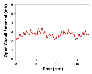
Figure 7. Typical Chronopotentiogram Acquired when Testing Reference Electrodes
