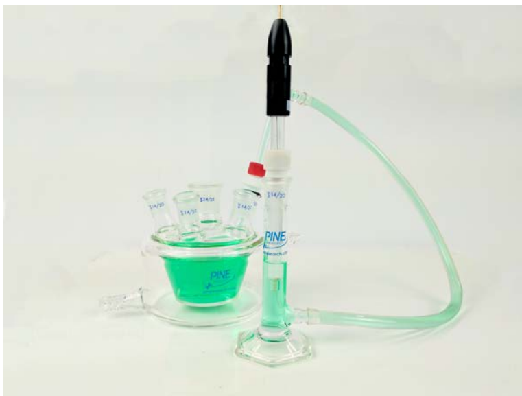
Figure 8. Complete Reference Electrode Setup with a Salt Bridge
