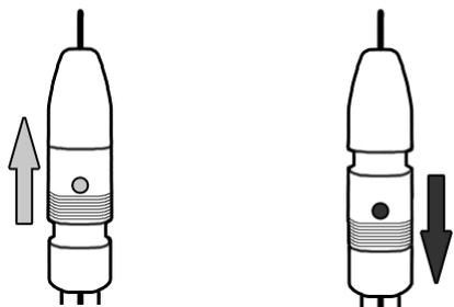
Slide access door (D) up to close the fill port for storage
