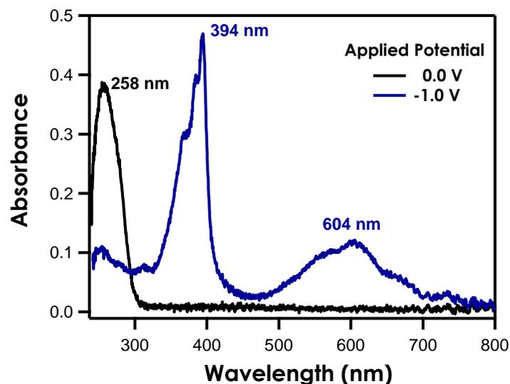
Figure 6-5. Absorption Spectra of  $MV^{2+}$  (black trace) and  $MV^{+\bullet}$  (blue trace)
