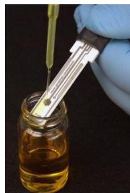
**Figure 5-3. Fill the Holes with Solution**
