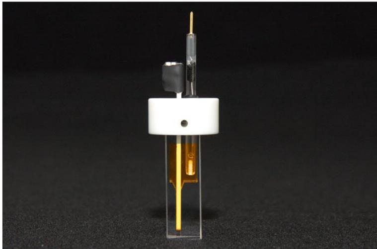
**Figure 5-4. Fully Assembled Honeycomb Spectroelectrochemical Cell with Solution**
