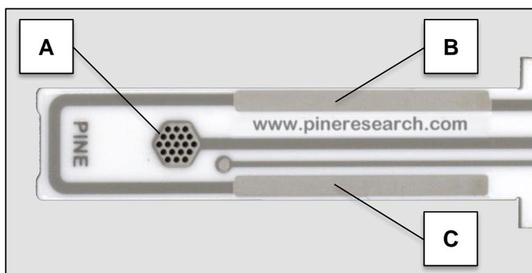
**Figure 2-2. Location of Working and Counter Electrodes**
