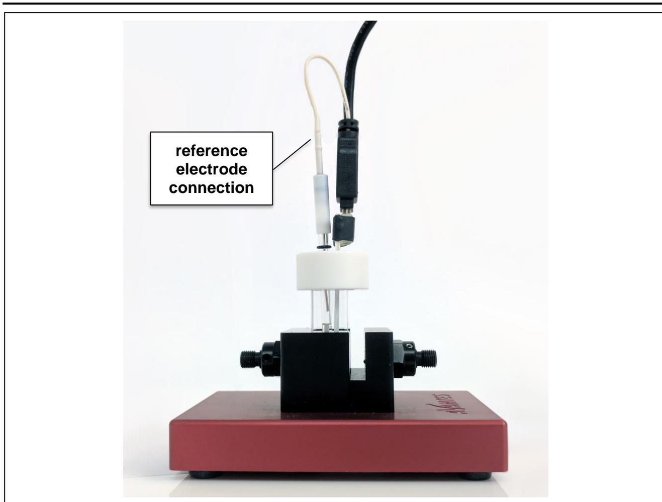
Figure 5-7. Connection to the Electrode Card and the Reference Electrode
