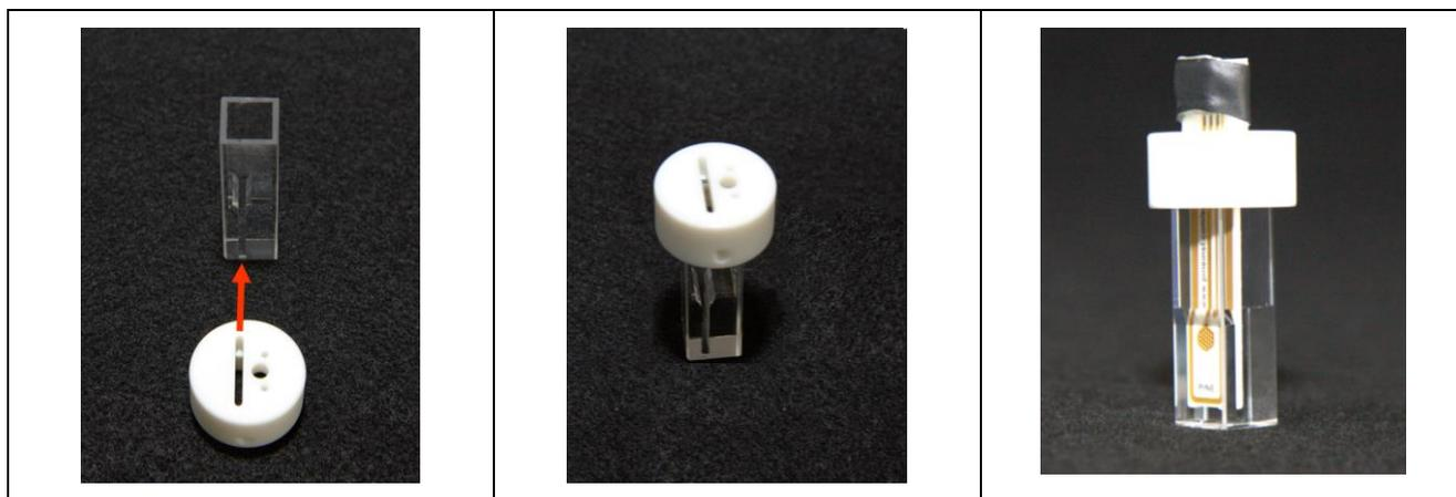
Figure 5-1. Proper Slot Alignment for the Quartz Cuvette, the Cap, and the Electrode Card
