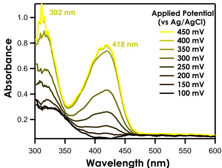
Figure 6-4. Absorption Spectra for the Ferricyanide/Ferrocyanide Redox Couple at Various Potentials
