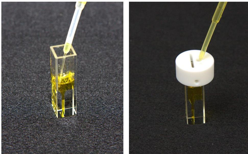
**Figure 5-2. Filling the Quartz Cuvette with Solution**
