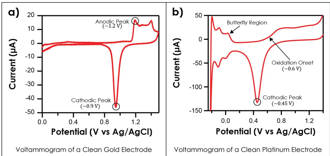
Figure 7-1. Characteristic Voltammograms for Clean Honeycomb Electrode Cards
