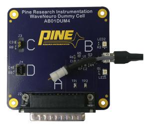
Figure 5-13. Connection of Headstage Cable to Dummy Cell B Connector
