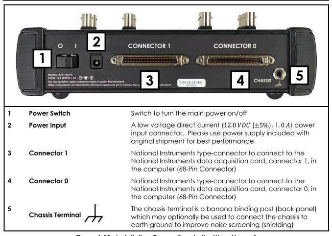
Figure 4-10: Installation Connections to the WaveNeuro 4
