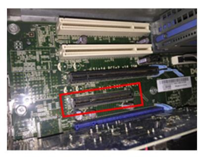
Figure 4-6: PCle Slot (Red Rectangle) on a PC Motherboard
