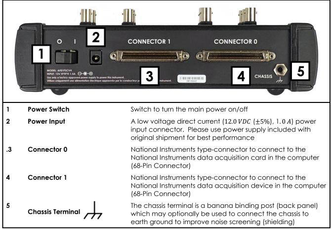
Figure 2-3: Description of the WaveNeuro 4 Side/End Panel
