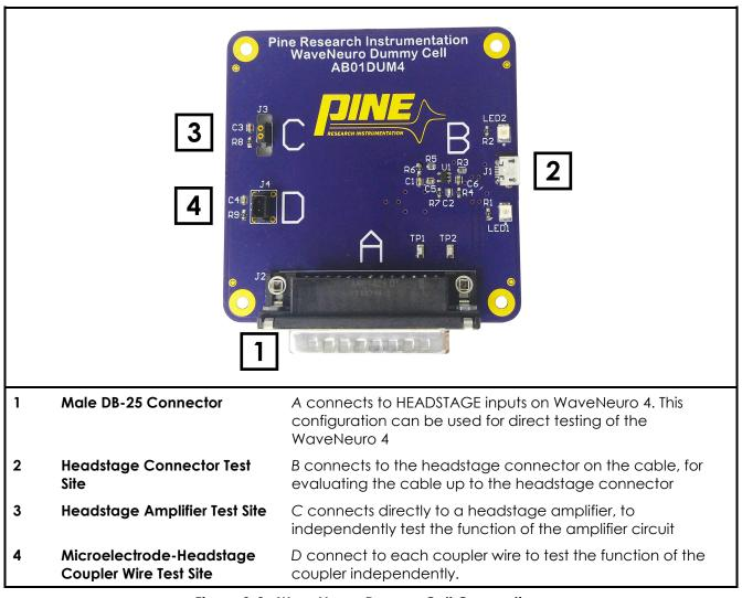
Figure 3-3: WaveNeuro Dummy Cell Connections
