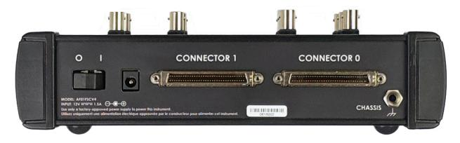
Figure 1-1: WaveNeuro 4 Side/End Panel Markings
