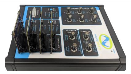
Figure 5-10: Connection of Four Dummy Cells to the WaveNeuro 4 HEADSTAGE Connectors
