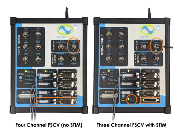
Figure 6-14: Unique Multichannel Configurations of the WaveNeuro 4
