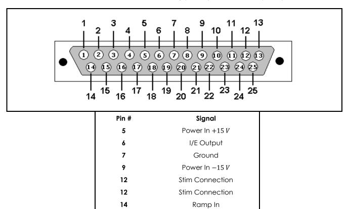
Figure 3-2: Headstage Cable DB-25 Connector Pinout Diagram
