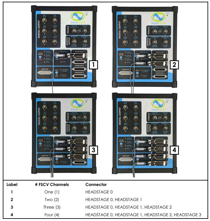
Figure 6-1: Multichannel Headstage Cable Installation for WaveNeuro 4
