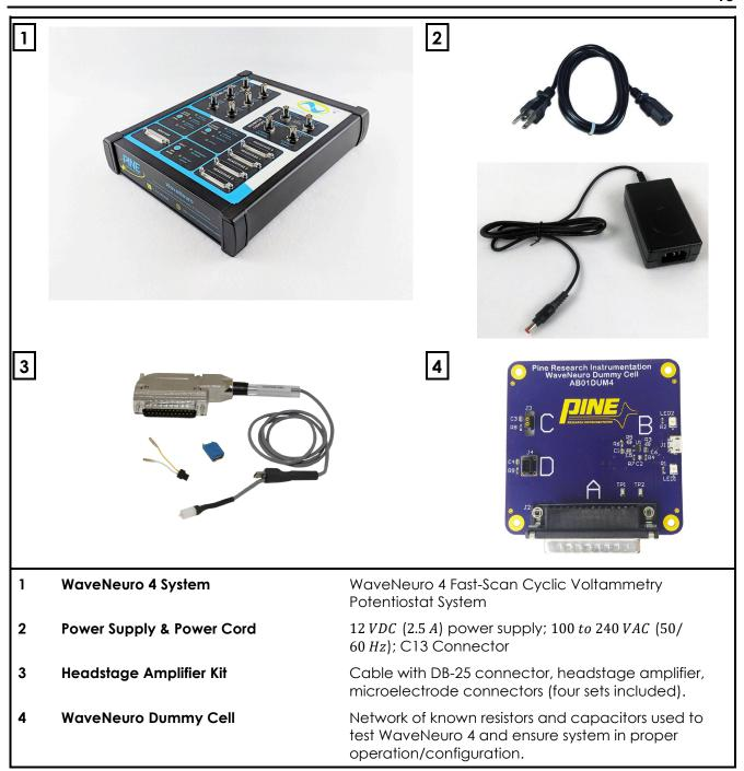
Figure 2-2: Major WaveNeuro 4 System Components (not to scale)
