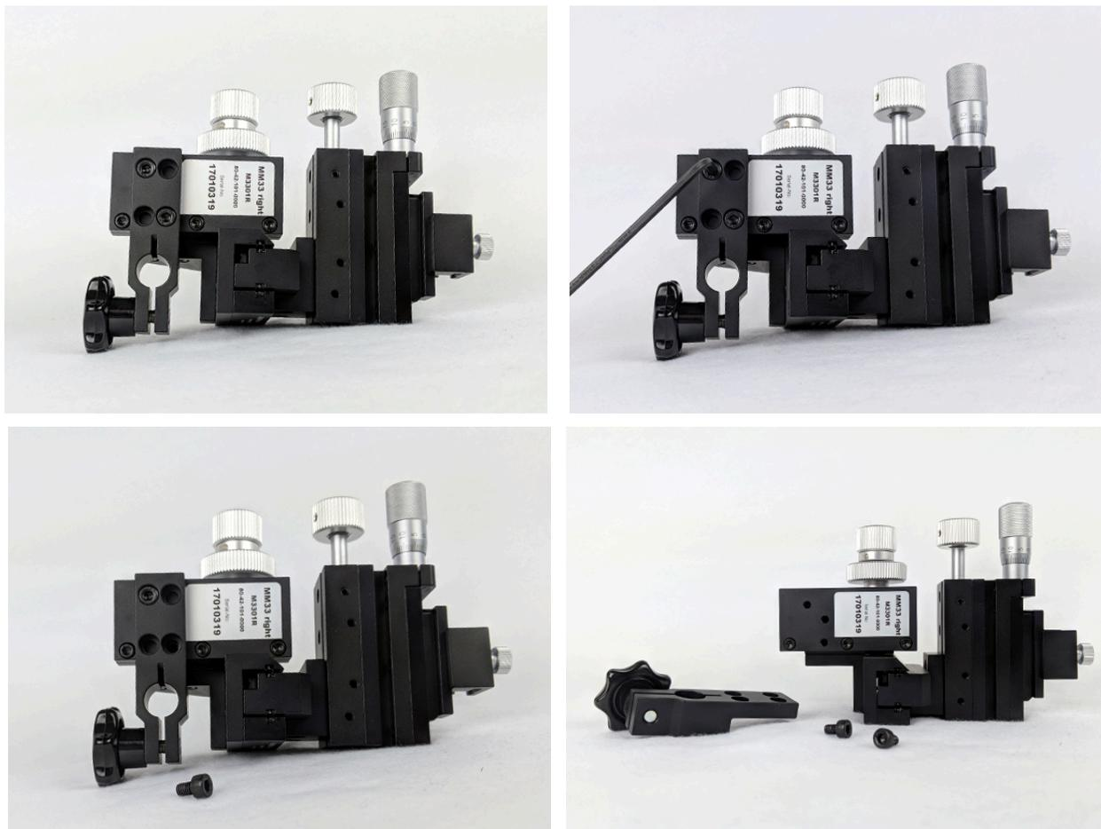
**Figure 3-12. Removal of Micromanipulator Bracket**
