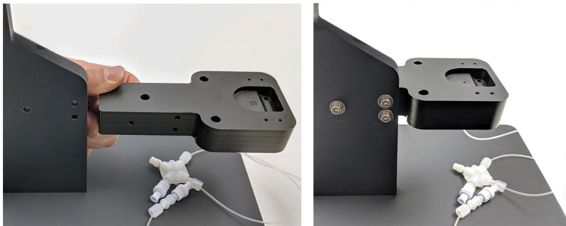
**Figure 3-11. Attachment of Flow Cell Body to Arm**
