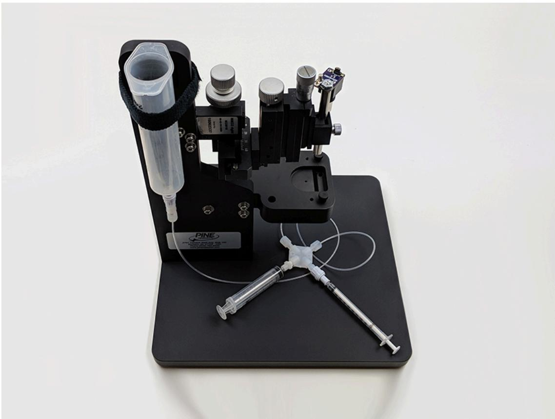
**Figure 4-10. Fully Assembled Flow Cell**
