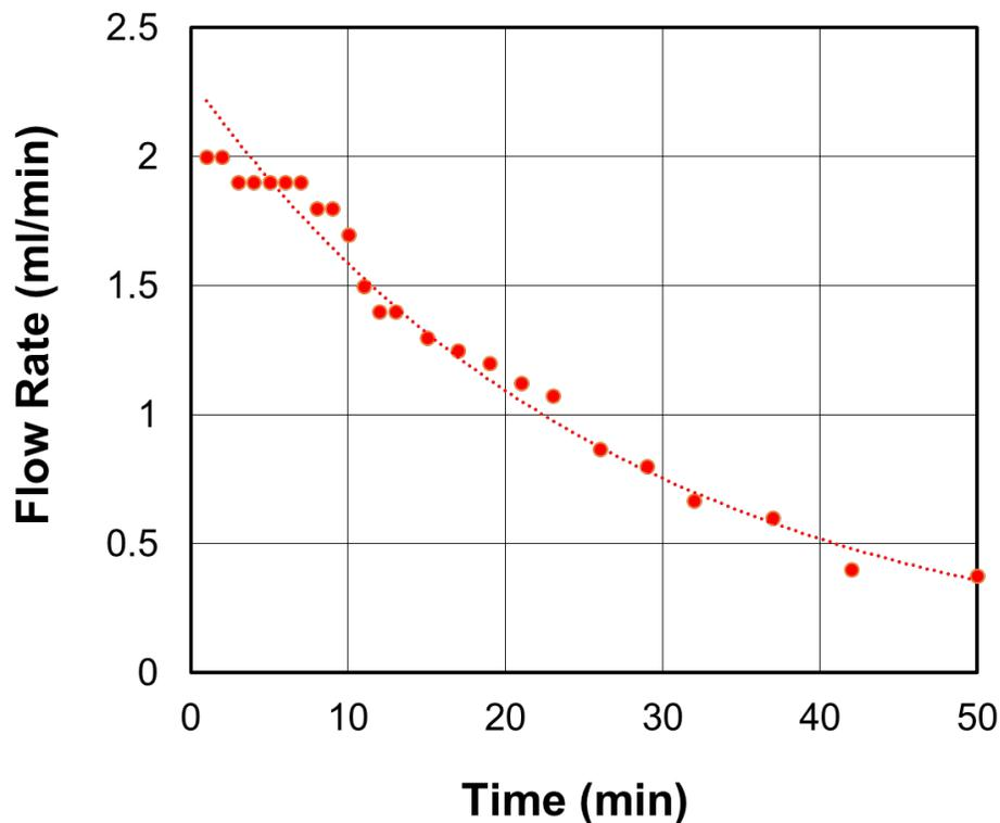
Figure 2-1. Gravity Feed Flow Rate Performance (dashed line running average)
