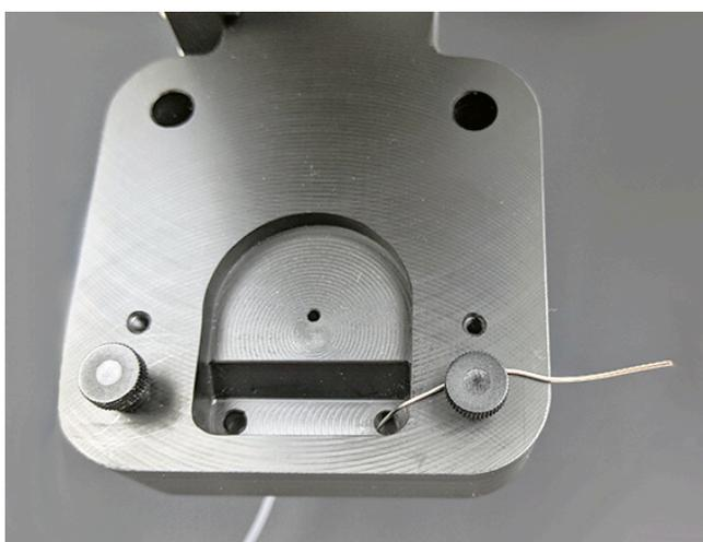
Figure 4-1. Reference Electrode Connection/Installation in Flow Cell
