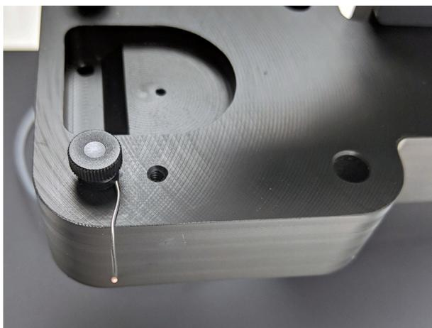
Figure 2-5. External Lead Thumb Screw Securing Reference Electrode Lead
