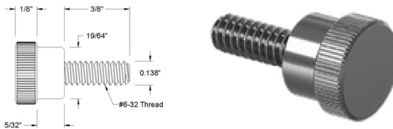
**Figure 2-4. Black Plastic External Lead Thumb Screw**
