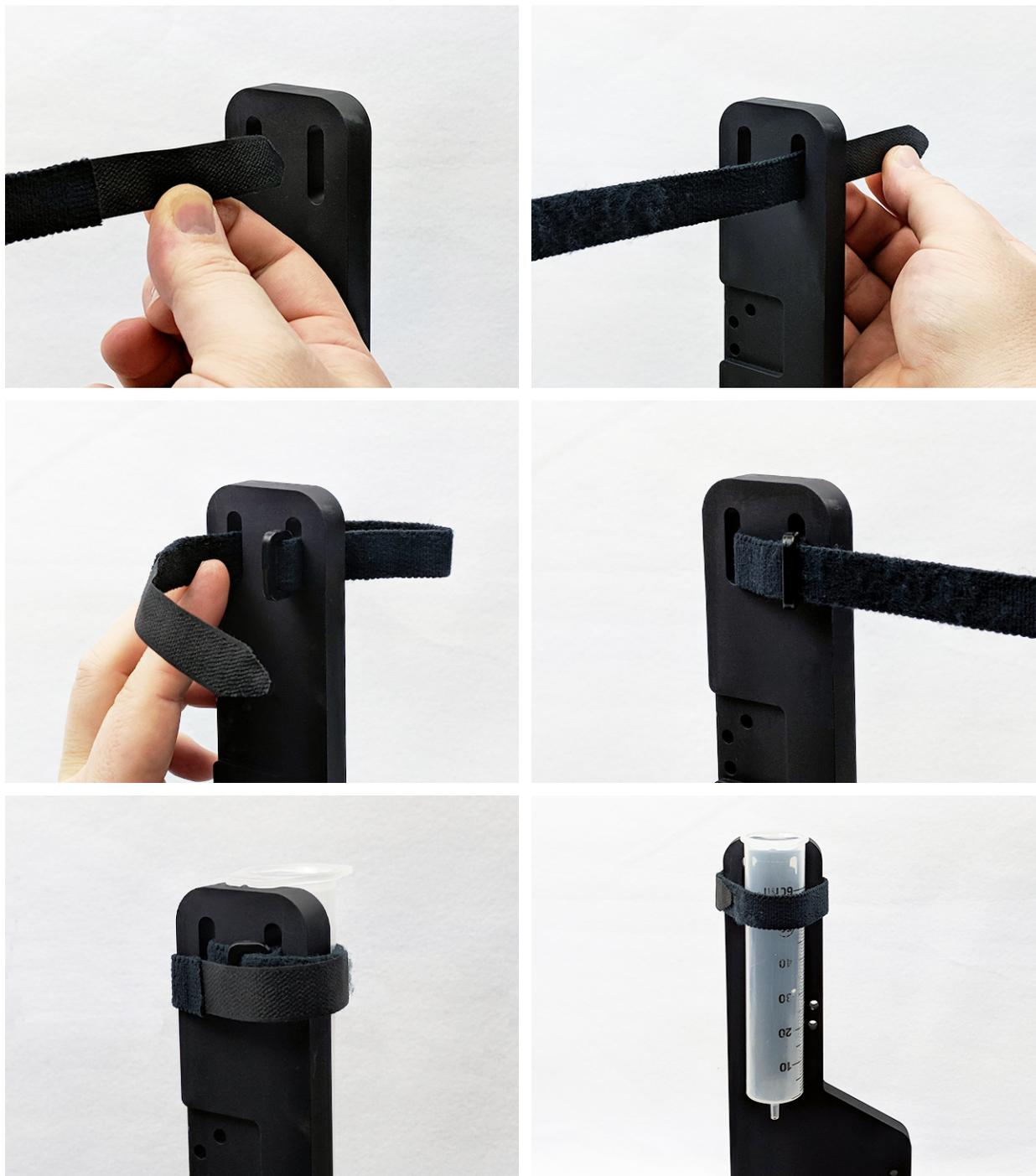
**Figure 3-9. Attachment of Buffer Reservoir Strap (left to right, top to bottom)**
