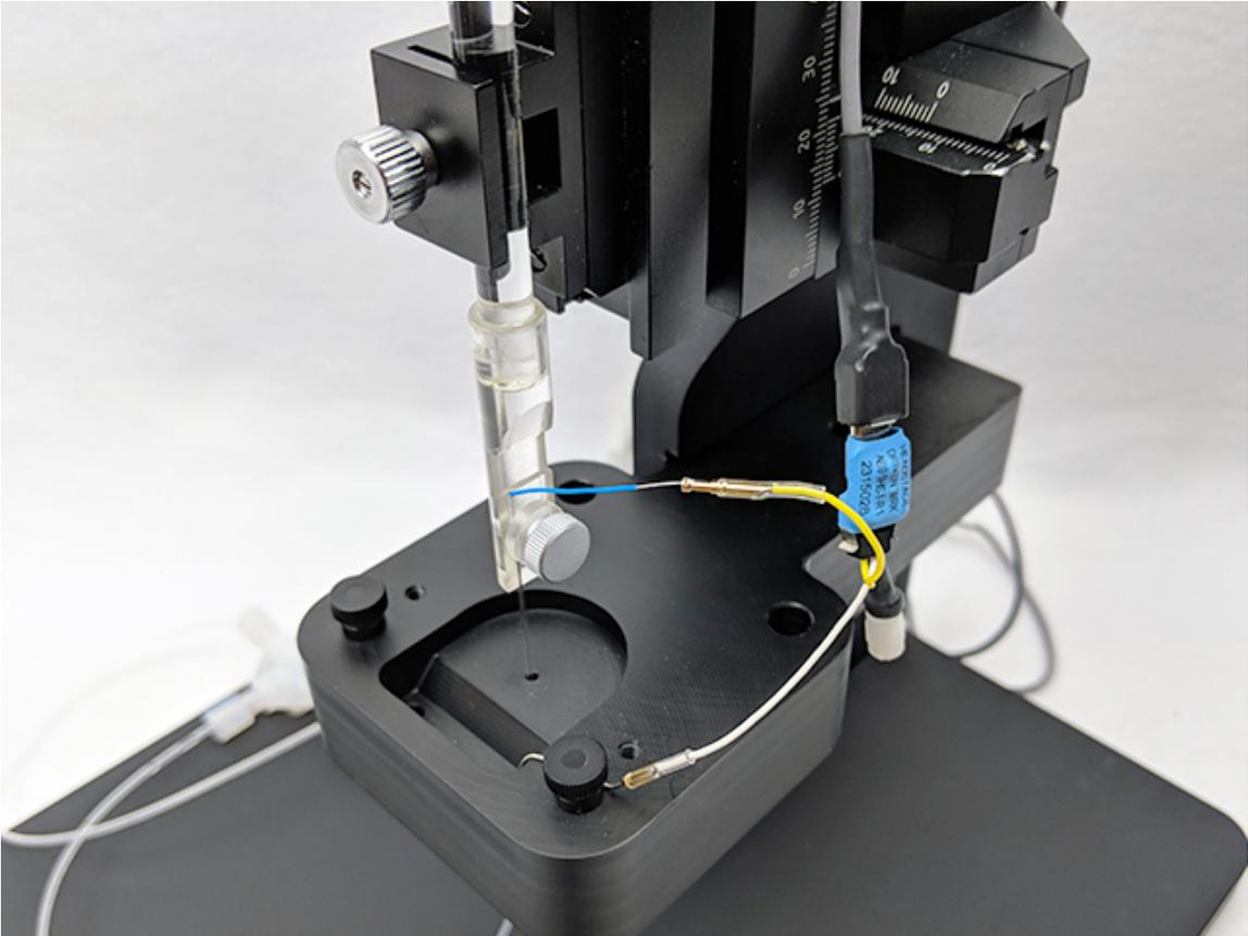
**Figure 4-4. Complete Electrode Holder Style Setup**
