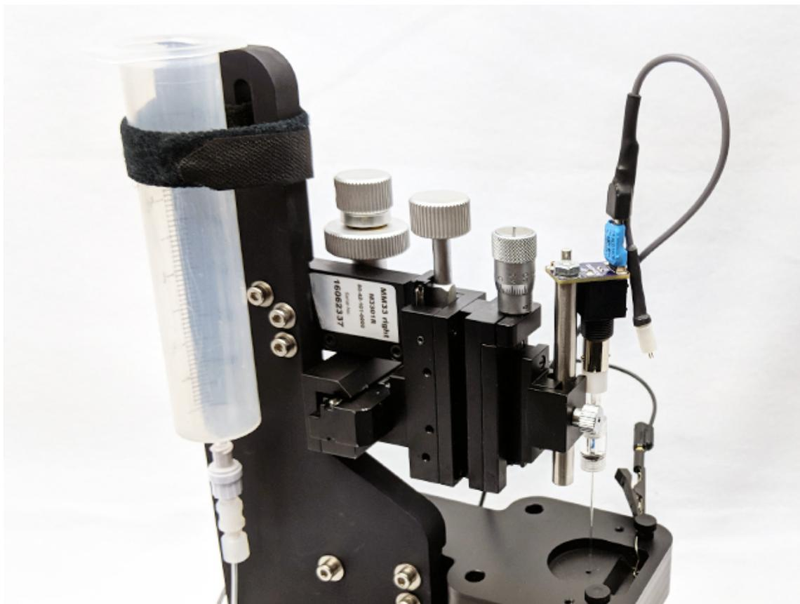
Figure 4-9. Fully Installed CFME in Using Malli Adapter in Micromanipulator
