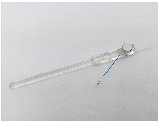
**Figure 4-2. Installation of Microelectrode into Micromanipulator Electrode Holder**
