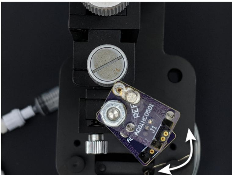
Figure 4-7. Mali Adapter for Flow Cell Variable Position
