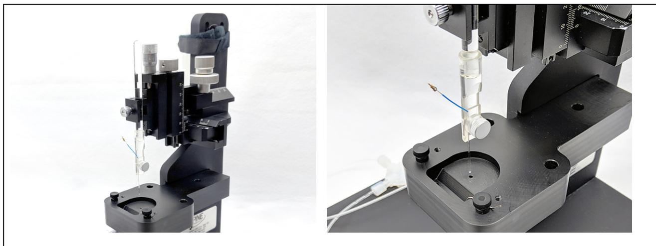
**Figure 4-3. Installation of Microelectrode Holder into Micromanipulator**
