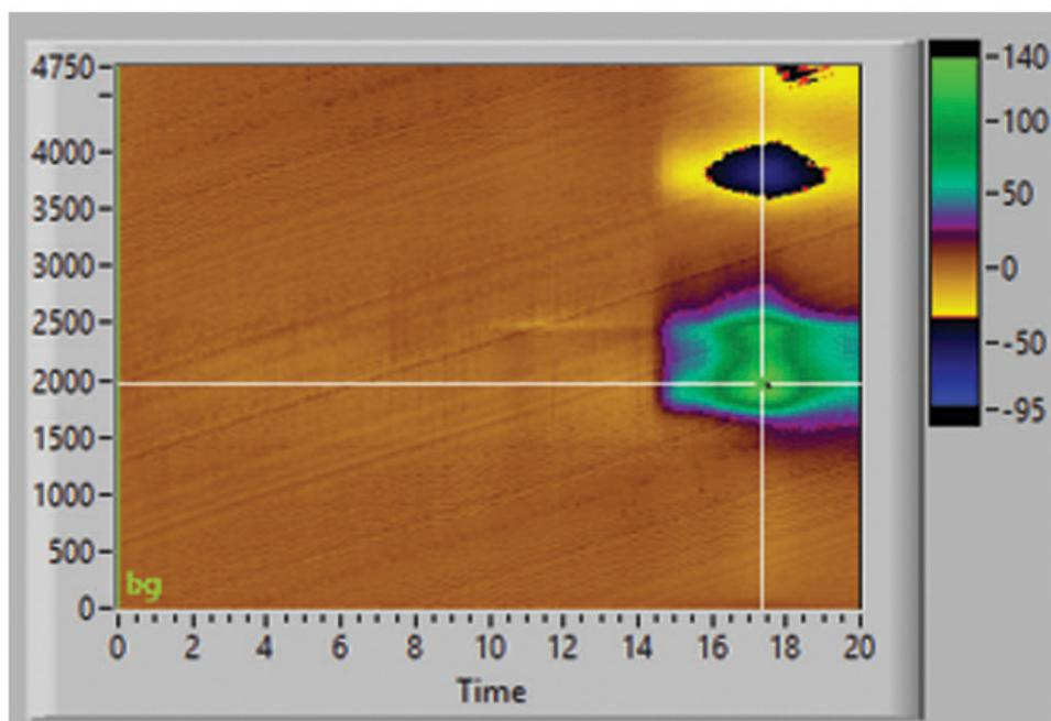
Figure 4-11. FSCV of 5-Hydroxytryptophan using Pine Research Flow Cell
