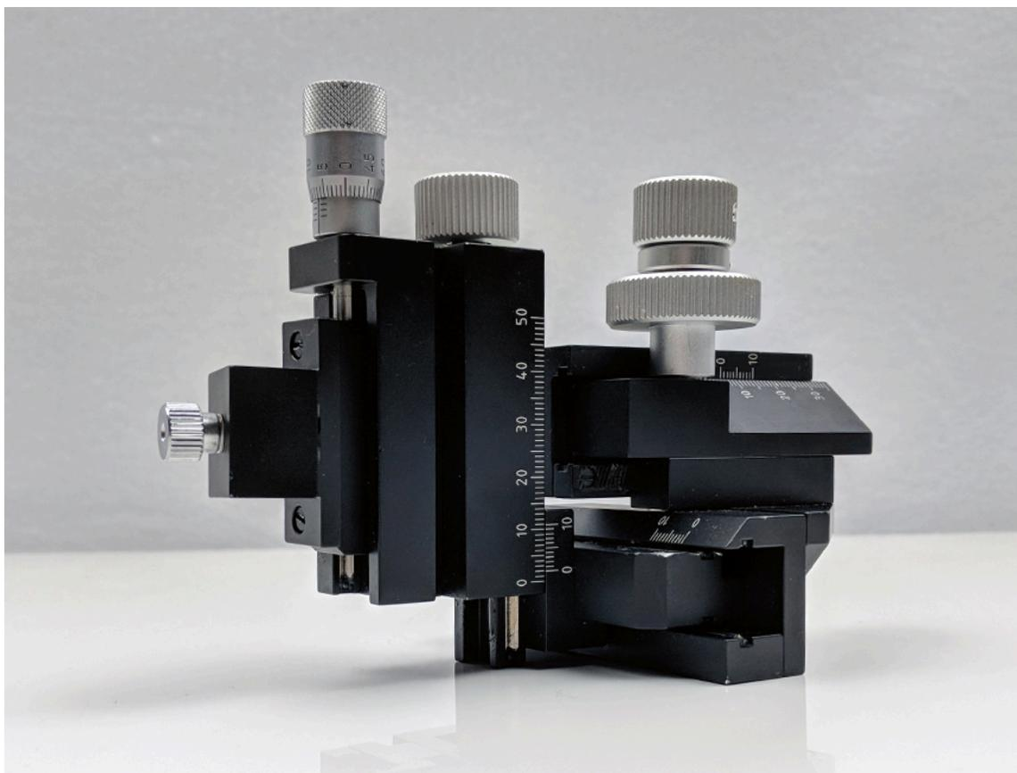
Figure 2-7. Optionally Available Micromanipulator (xyz Translational Stage)
