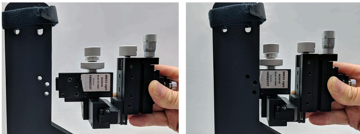
Figure 3-13. Attachment of the Micromanipulator to Arm
