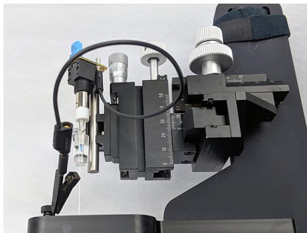
Figure 4-8. Connecting Electrodes to Potentiostat on a Mali Adapter for Flow Cell
