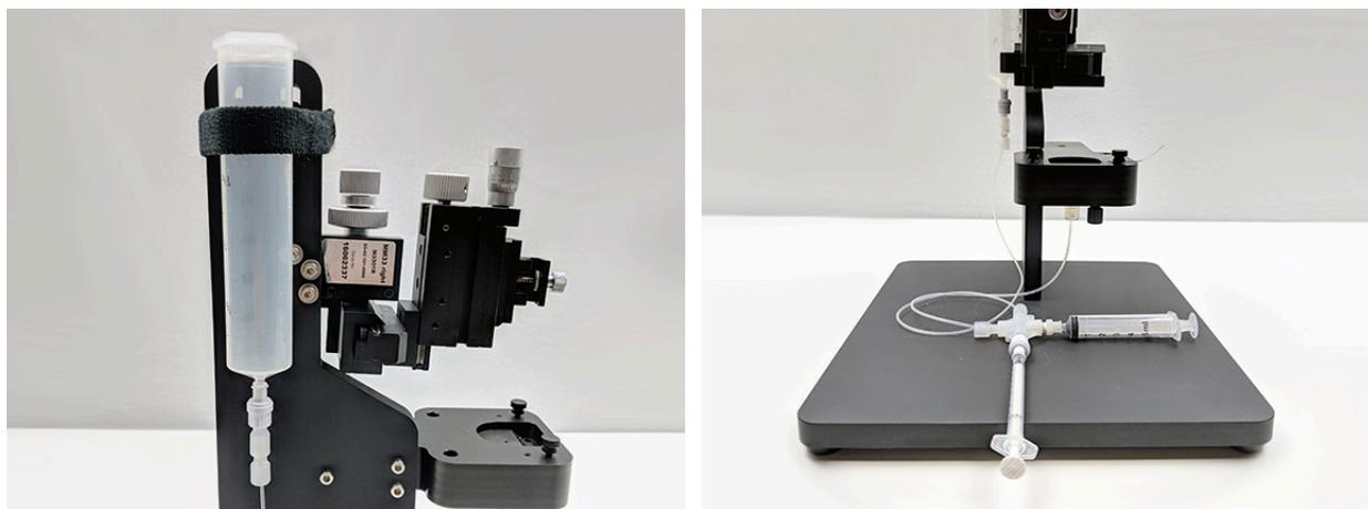
Figure 3-14. Completed Fluidic and Mechanical Assembly of Flow Cell
