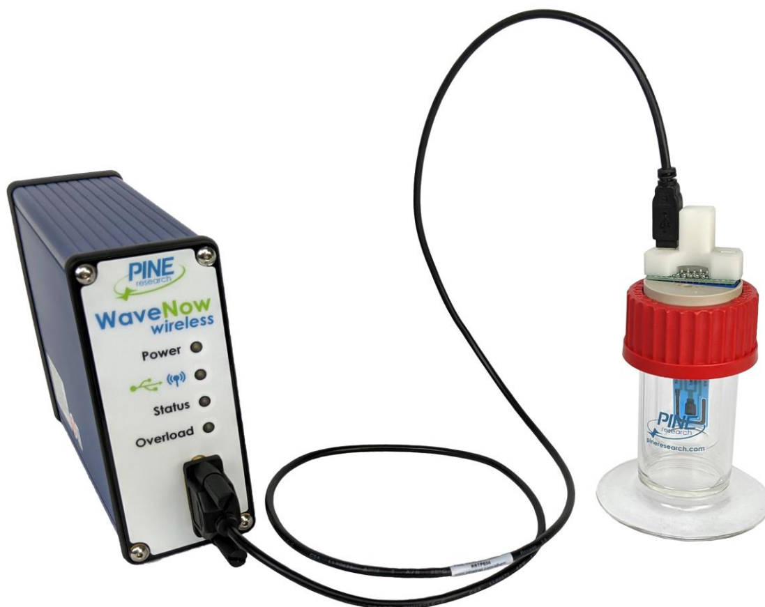
Figure 5-8. Cable Connections for the Compact Voltammetry Cell Kit
