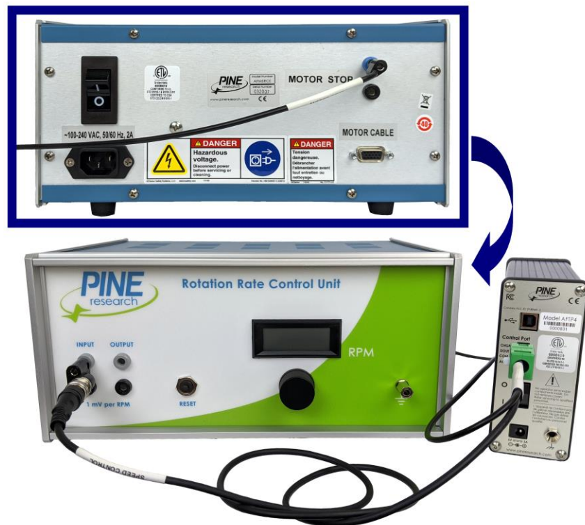
Figure 5-6. Rotation Rate Control Connections for a Pine Research MSR Rotator
