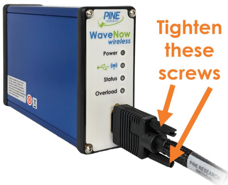
Figure 5-1. Secure Connection of WaveNow/WavePico Wireless Cell Cable to Cell Port
