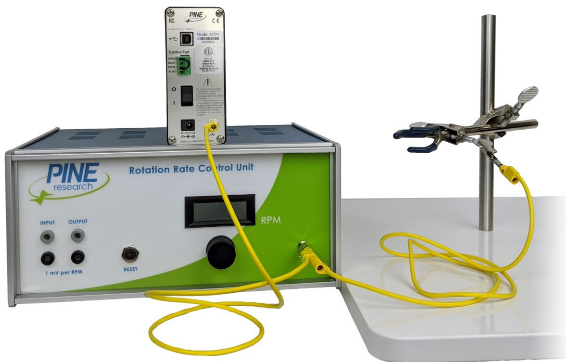
Figure 6-6. Connect All Instrument Chassis Terminals to a Common Point
