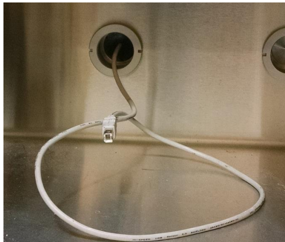
Figure 3-1. USB Cable Glovebox Feedthrough
