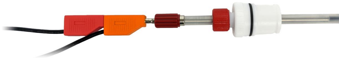
Figure 5-3. Working Electrode Sense and Drive Lines Shorted Together near the Electrode
