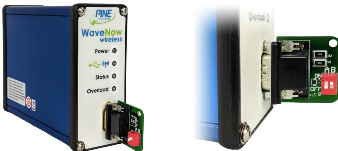
Figure 4-5. WaveNow Wireless Connected to Dummy Cell with 49.9 k \Omega Resistor Setting
