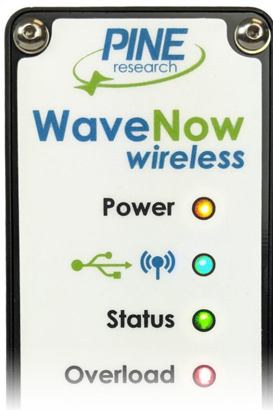
Figure 3-18. Instrument Light Status during Hardwired USB Connection (Blue-Green)
