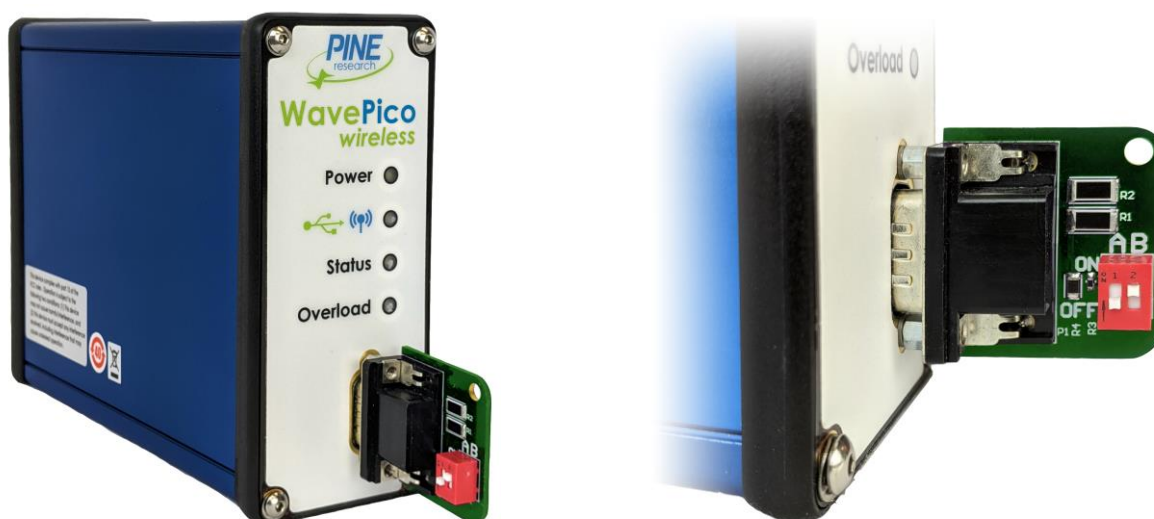
Figure 4-11. WavePico Wireless Connected to Dummy Cell with 4.99 M \Omega Resistor Setting
