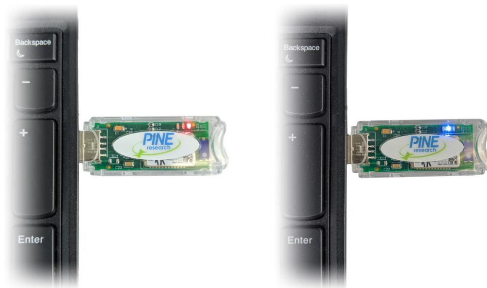
Figure 3-19. Wireless USB Dongle Indicating Connection Status (Red or Blue)
