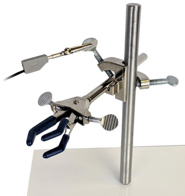
Figure 6-4. Metal Objects Near the Electrochemical Cell Should Be Grounded
