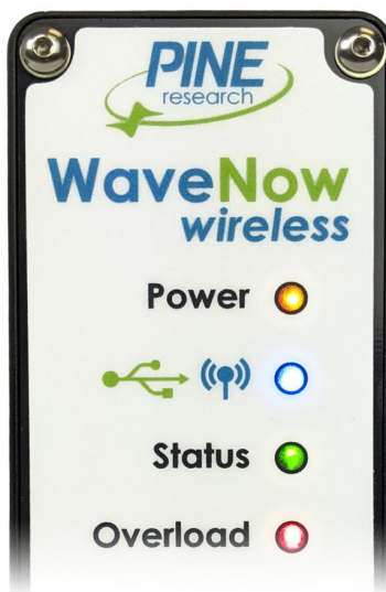
Figure 4-3. Indicator Lights on the Front Panel of the WaveNow Wireless
