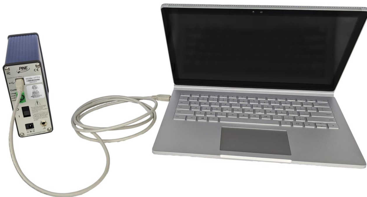
Figure 3-17. USB Cable Connection Between Potentiostat and Computer
