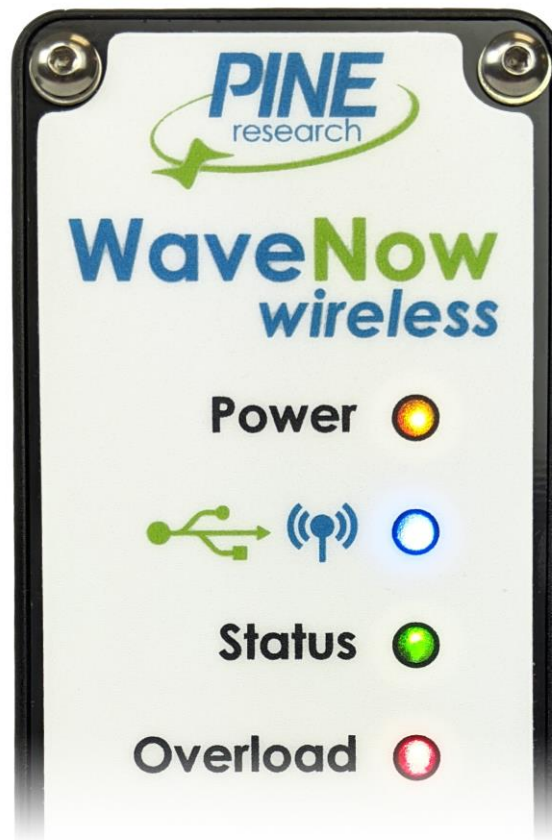
Figure 3-20. Instrument Light Status during Wireless Connection (Blue)
