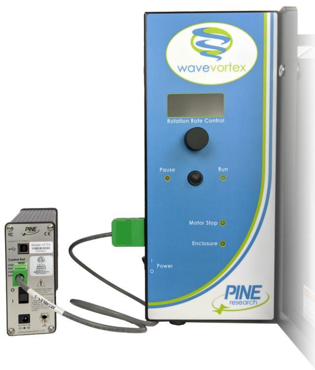
Figure 5-7. Rotation Rate Control Connections for a Pine Research WaveVortex 10 Rotator
