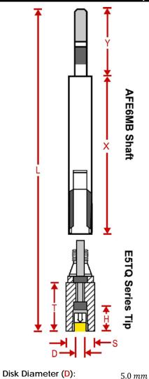
Shroud Diameter (S): 15.0 mm Tip Shroud Length (T): 25.4 mm Overall Length (L): 196.9 mm Upper Shaft Length (Y): 69.9 mm Lower Shaft Length (X):  $100.8 \ mm$
