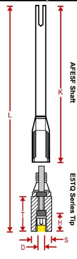
Disk Diameter (D): 5.0 mm Shroud Diameter (S): 15.0 mm Tip Shroud Length (T): 25.4 mm Overall Length (L): 184.2 mm Shaft Length (K): 158.0 mm Max. Immersion (H):
