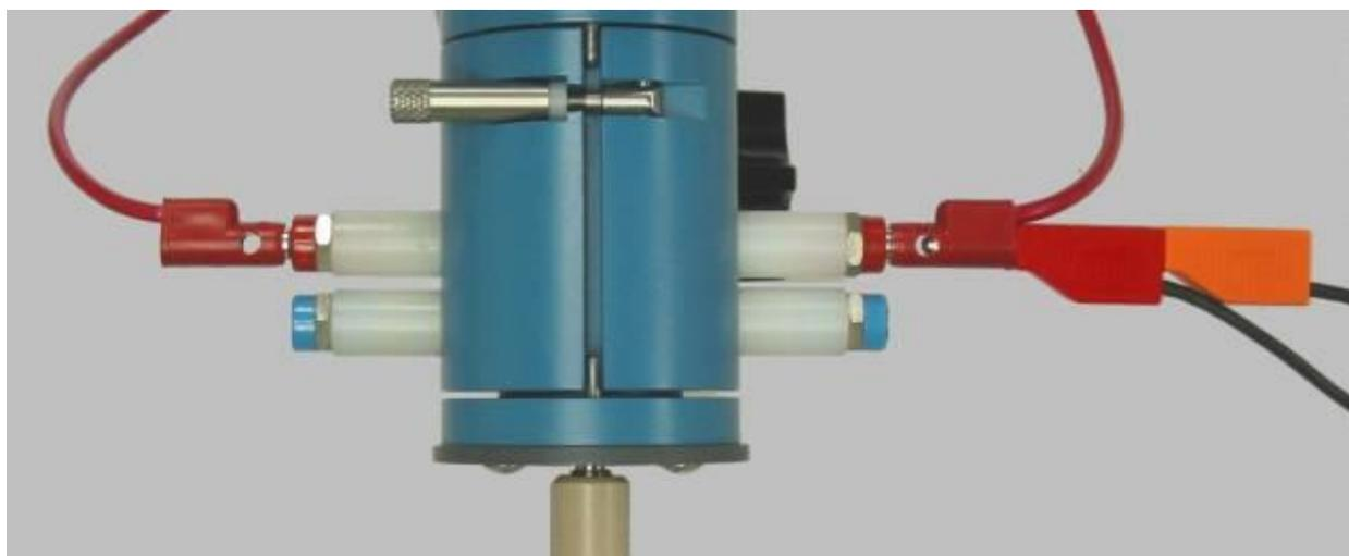
Figure 5-7. Working Electrode Connections for Rotating Disk or Cylinder Electrodes
