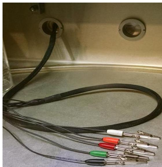
**Figure 3-2. Cell Cable Glovebox Feedthrough**
