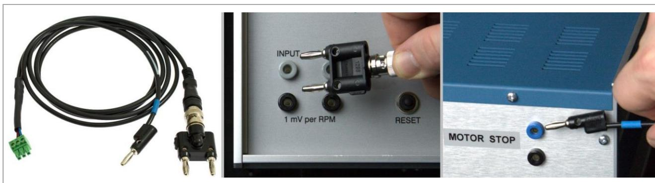
Figure 5-9. Rotation Rate Control Between WaveDriver and MSR Rotator
