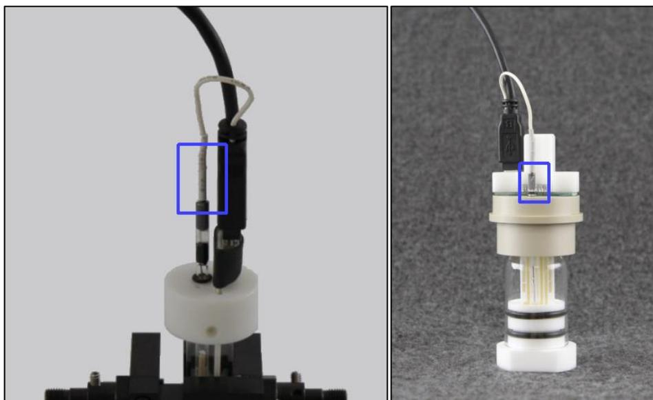
**Figure 5-11. Compact Voltammetry and Spectroelectrochemical Cells with Separate Reference Electrode Connections**
