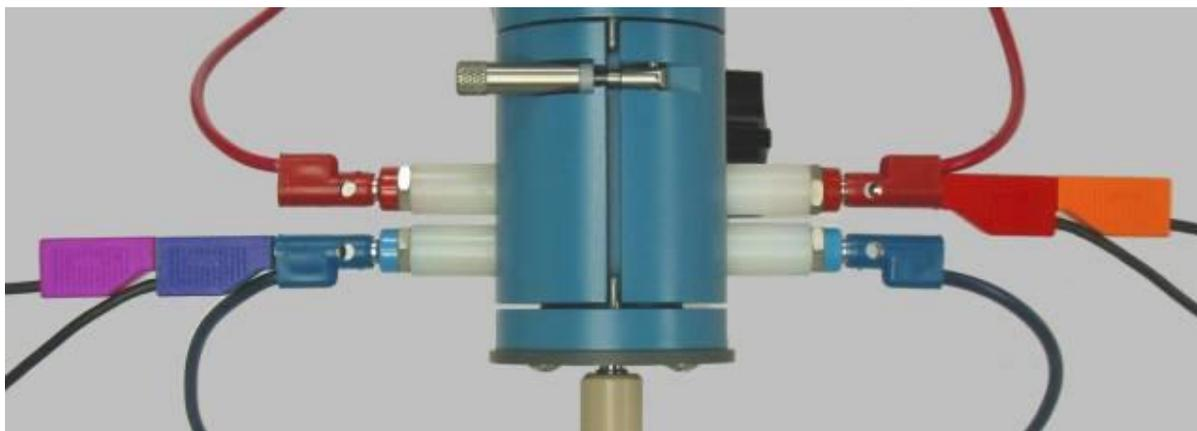
Figure 5-8. Electrode Connections (K1 and K2) for a Rotating Ring-Disk Electrode
