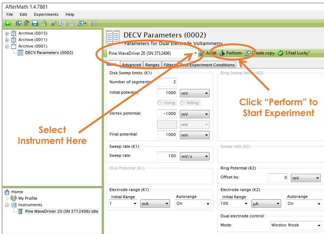
Figure 4-11. Location of Instrument Selection menu and Perform button (DECV)
