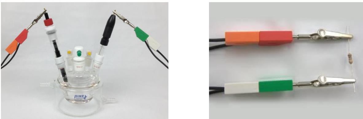
**Figure 5-3. Examples of Two-Electrode Cells**
