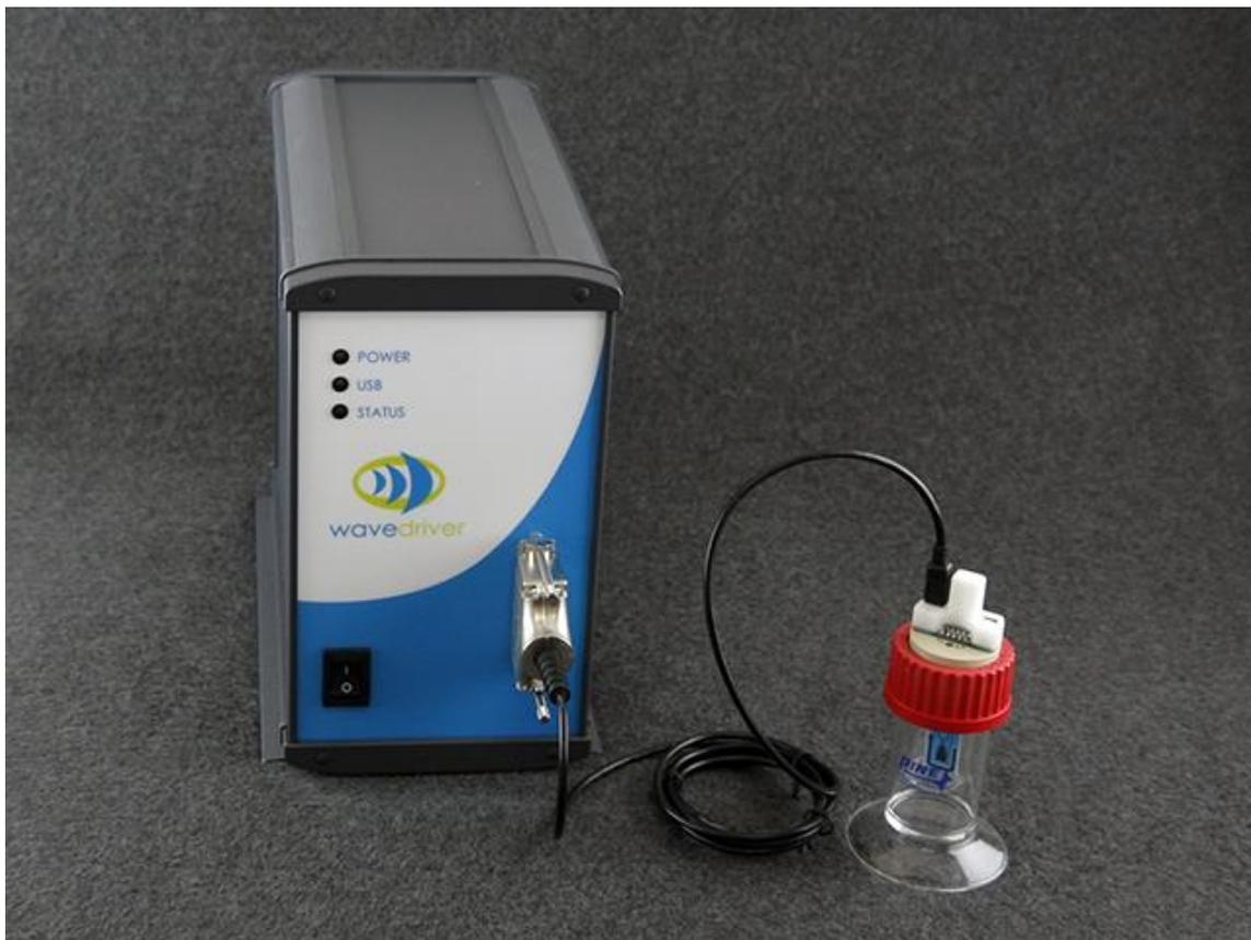
Figure 5-10. Cable Connections for the Compact Voltammetry Cell Kit
