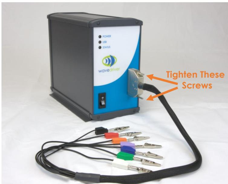
**Figure 5-2. Securely Tighten the D-Shell Connector to the Cell Port**
