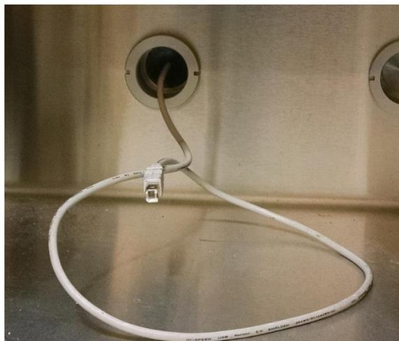
**Figure 3-1. USB Cable Glovebox Feedthrough**
