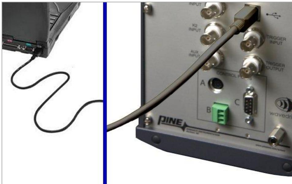
Figure 3-4. USB Cable Connection between WaveDriver Potentiostat and Computer
