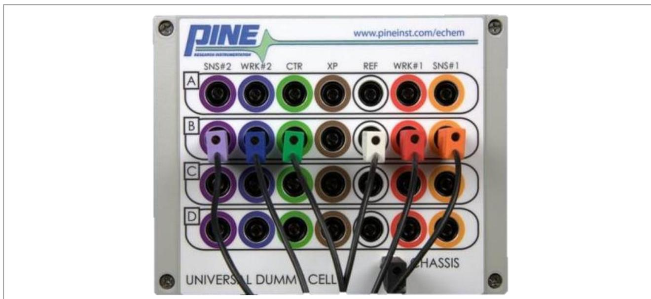
Figure 2-6. Universal Dummy Cell Connected to the WaveDriver 20
