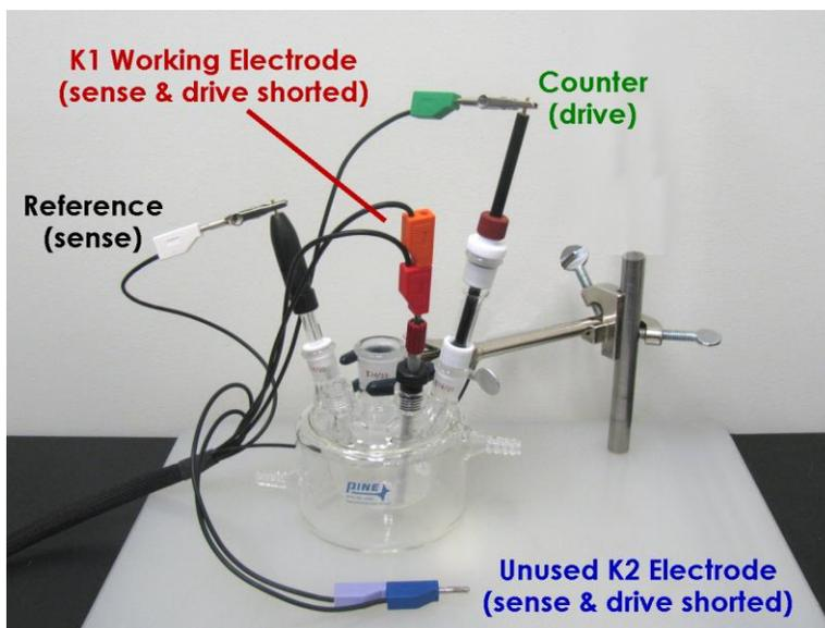
**Figure 5-5. Traditional Three-Electrode Cell Connections**
