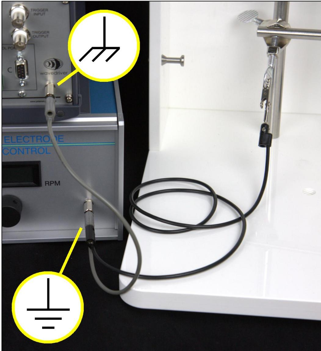
Figure 6-2. Ground Multiple Instruments and Objects to a Common Point
