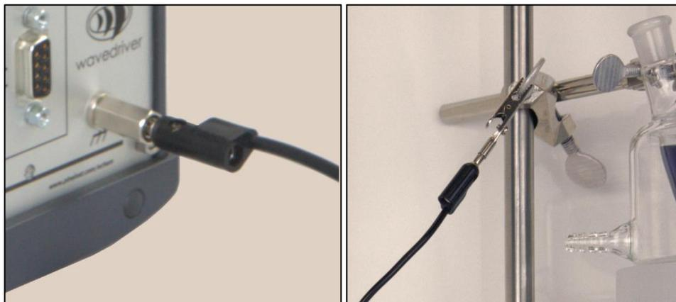
**Figure 6-1. Connect Clamps and Other Metal Objects to Instrument Chassis and/or Earth Ground**
