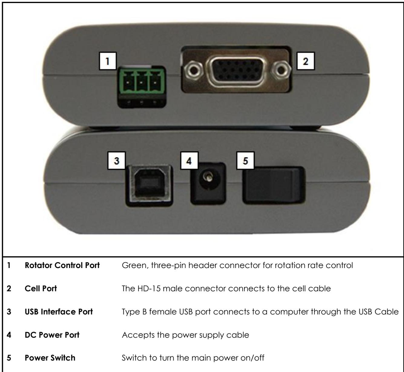
Figure 2-2. The Side Panels of the WaveNow, WaveNano, and WaveNow<sup>XV</sup>
