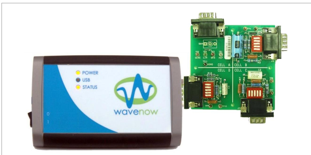
**Figure 2-5. Dummy Cell Connected to the WaveNow**
