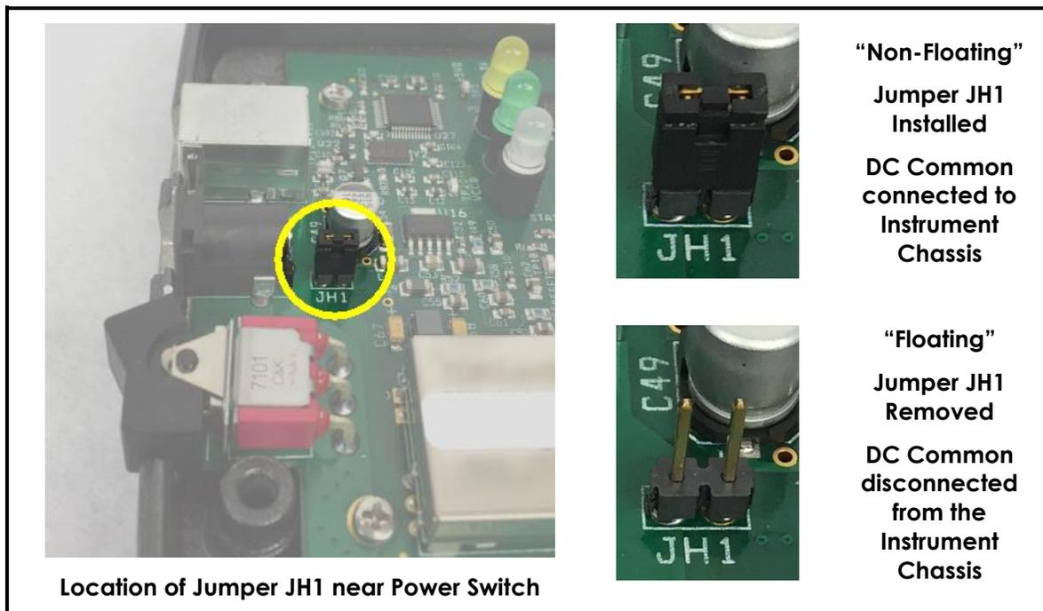
**Figure 6-1. Floating vs. Non-Floating DC Common Configuration**
