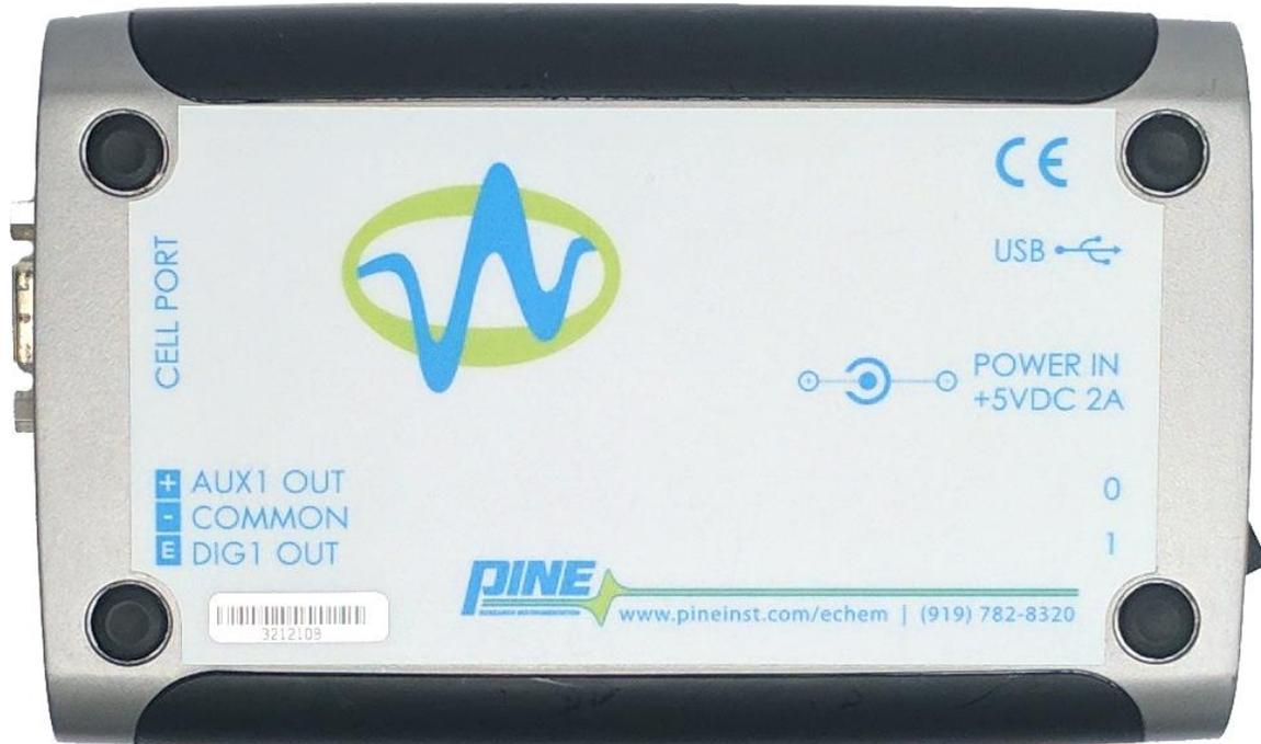
Figure 1-1. WaveNow, WaveNano, and WaveNow<sup>xv</sup> Bottom Panel Markings
