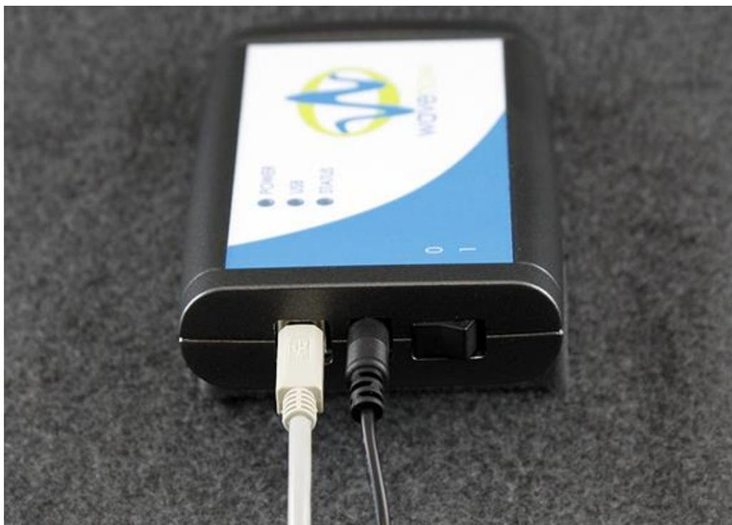
**Figure 3-5. USB Cable Connection between Potentiostat and Computer**
