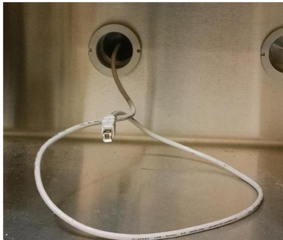
**Figure 3-1. USB Cable Glovebox Feedthrough**
