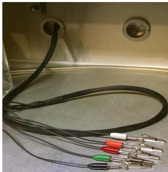
**Figure 3-2. Cell Cable Glovebox Feedthrough**
