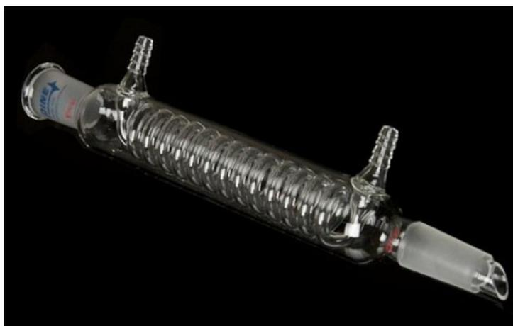
**Figure 18. 15mm RCE Cell Condenser, an Optional Accessory.**
