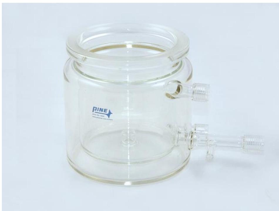
**Figure 11. The jacketed OpenTop 1 Liter Corrosion cell with drain.**
