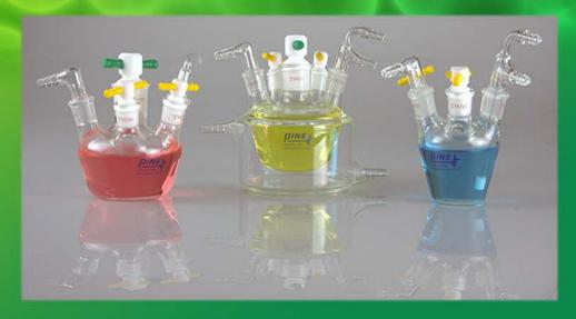
From traditional two-electrode H-cells to three-electrode cells to more advanced setups with custom dimensions, our glass cells are versatile with unmatched quality. Folks have trusted us to design their own custom cells for years. Our cells integrate seamlessly with our electrodes (stationary and rotating) and adapters. We are not limited to electrochemical cells. Discuss your application with us today and we will be happy to work with you.
