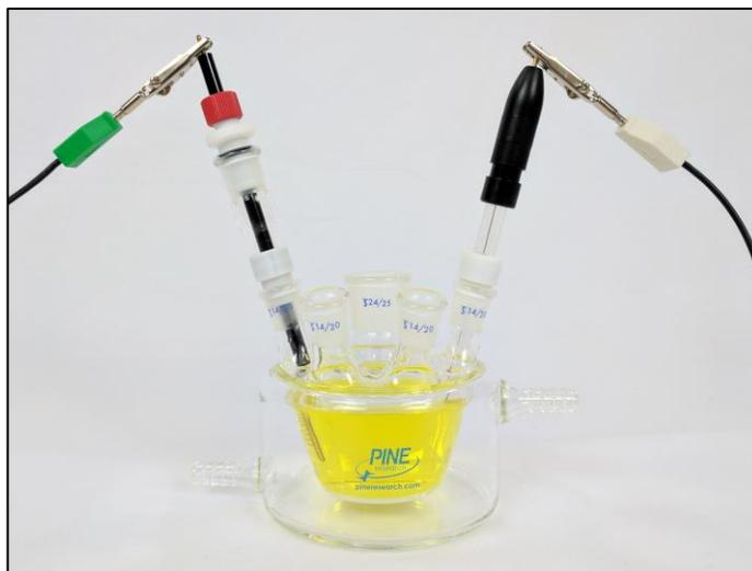
**Figure 4-12. Connection of Counter and Reference Electrodes**
