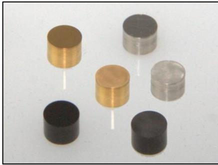
The standard size of a disk insert is 5 mm OD × 4 mm thick. Pine Research offers many types of disk materials, including carbon materials, precious metals, steels and alloys, and other common metals. Most disk inserts are shipped from the production facility with a mirror polish.
