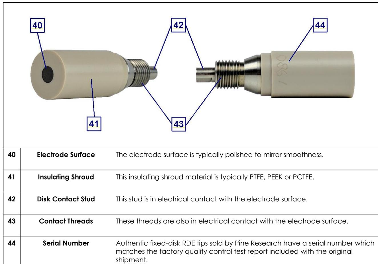
**Figure 2-6. Typical Rotating Disk Electrode (RDE) Tip**
