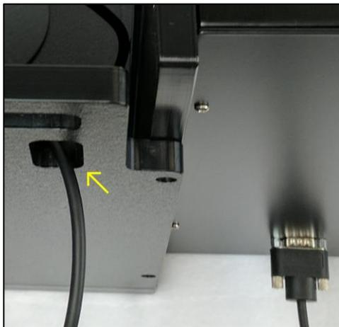
Feed the motor cable through the opening in the back wall of the cell enclosure.
