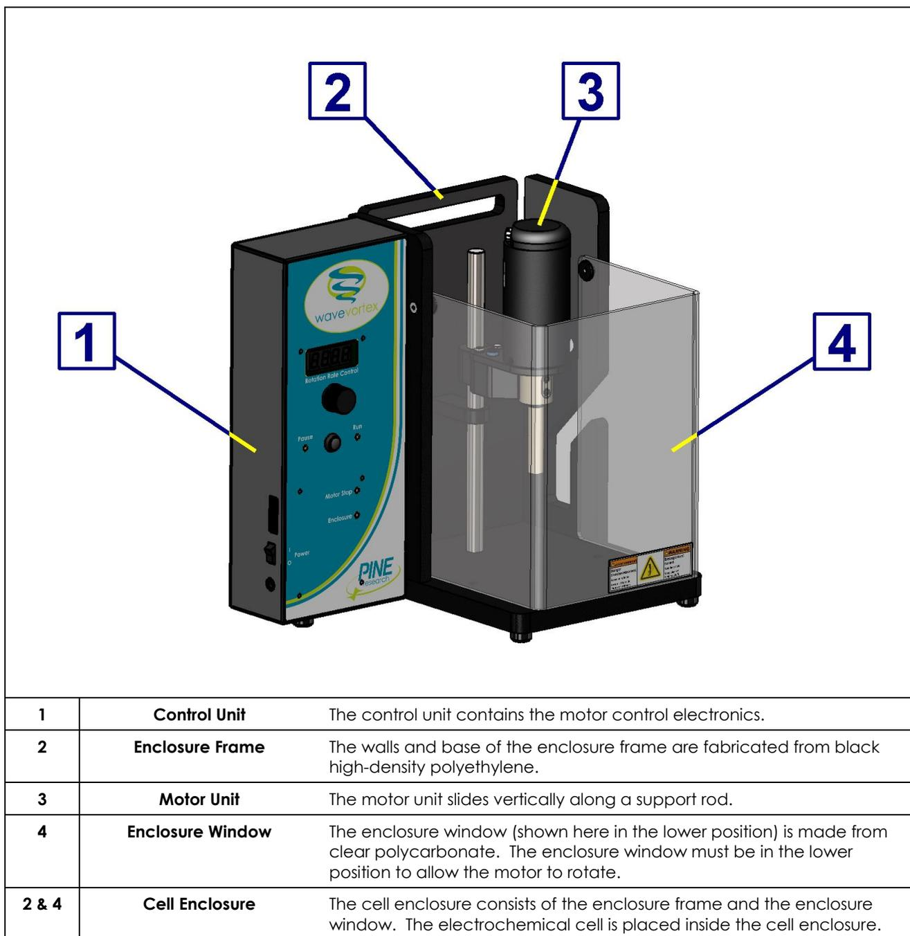
**Figure 2-1: Major Components of the WaveVortex Rotator System**
