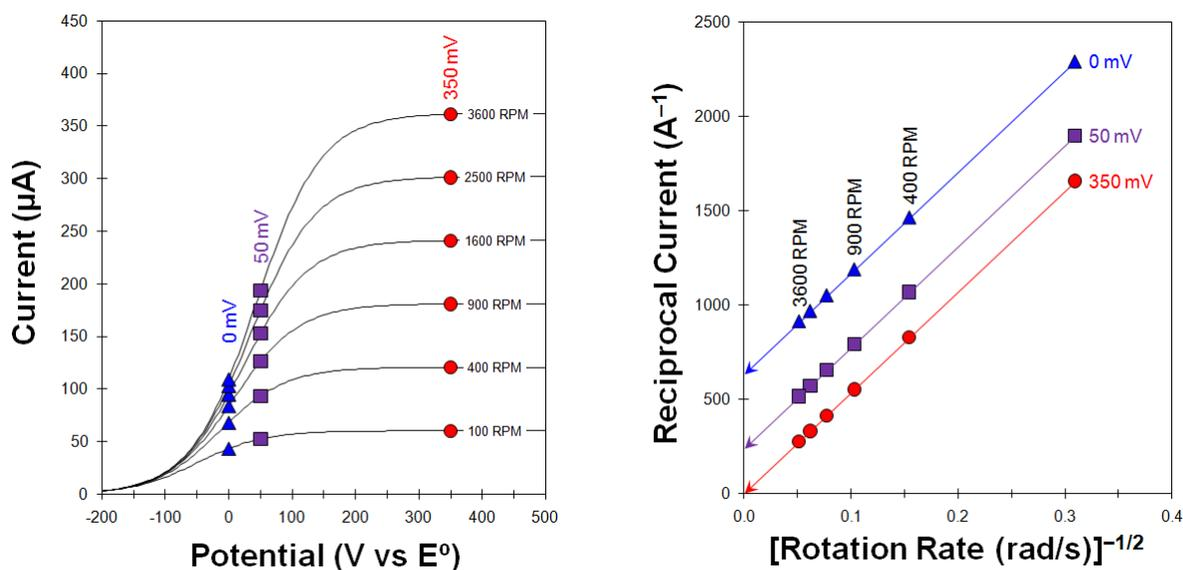
Figure 9-9. Koutecky-Levich Study – Voltammograms with Sluggish Kinetics
