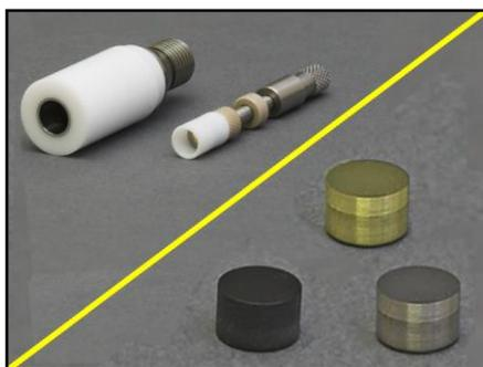
These RRDE tips feature a removable disk electrode surrounded by a ring electrode and a PTFE shroud. The disk insert is sold separately (see: Section 5.10), allowing the same ring electrode to be used with a variety of different disk materials. The seal between the disk and the ring (known as a “U-Cup”) is made from hydrophobic PTFE.
