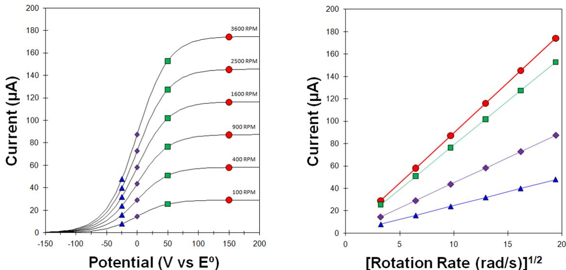
**Figure 9-7. Levich Study – Voltammograms at Various Rotation Rates**
