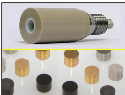
These RDE tips feature a 15 mm OD shroud around a 5 mm OD disk electrode. The disk insert is removable, and a variety of disk insert materials are available separately (see: Section 5.10).
