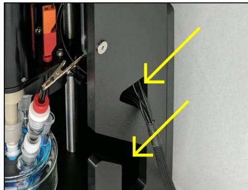
**Figure 4-6. Access Slots for Cables and Tubing**
