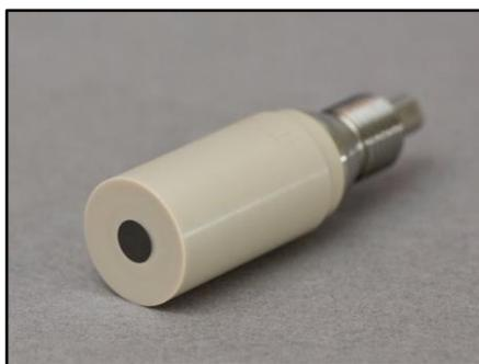
These RDE tips feature a 15 mm OD PEEK shroud around a 5 mm OD disk electrode. These tips fit the WaveVortex shaft and may be used at rotation rates up to 3000 RPM.
