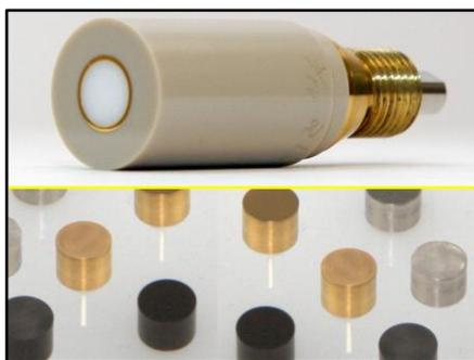
These RRDE tips feature a removable disk electrode surrounded by a ring electrode and a PEEK shroud. The disk insert is sold separately (see: Section 5.10), allowing the same ring electrode to be used with a variety of different disk materials. The seal between the disk and the ring (known as a “U-Cup”) is made from hydrophobic PTFE.
