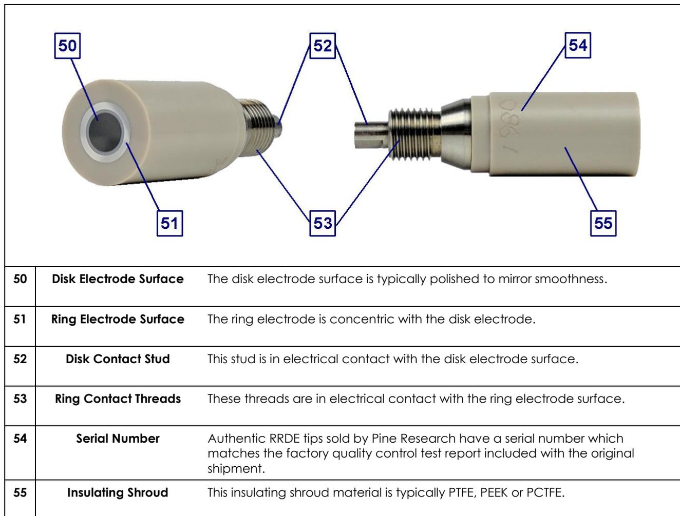
**Figure 2-7: Typical Rotating Ring-Disk Electrode (RRDE) Tip**
