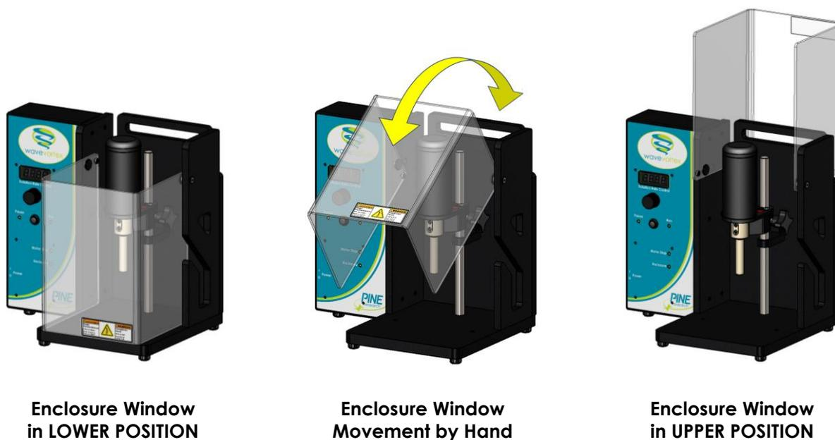
**Figure 4-1. Raising and Lowering the Enclosure Window**
