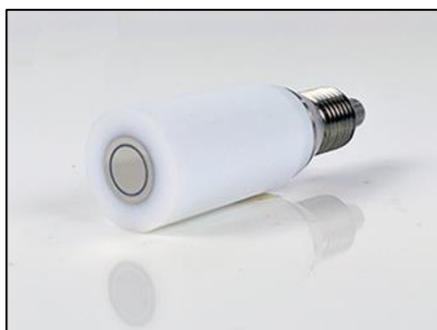
These RRDE tips feature a permanently mounted disk electrode surrounded by a ring electrode and a PTFE shroud. PTFE has excellent chemical resistance and abrades easily when hand-polishing the RRDE tip. The PTFE seal between the disk and the ring is very thin, allowing a short transit time for species travelling from the disk to the ring.
