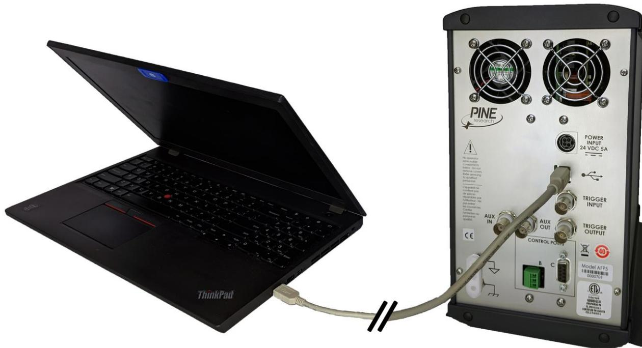
Figure 3-18. USB Cable Connection Between Potentiostat and Computer
