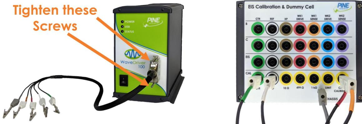
Figure 10-3. WaveDriver 100 Connections for Cell Cable Calibration
