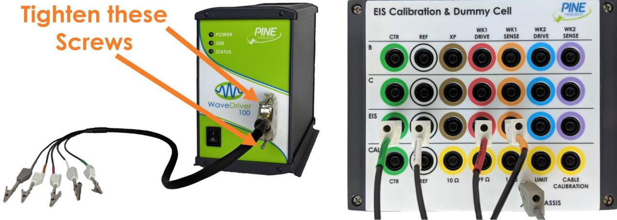
Figure 10-4. WaveDriver 100 Connections for a Simple EIS Test
