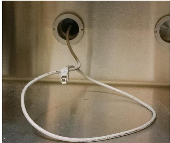
**Figure 3-1. USB Cable Glovebox Feedthrough**
