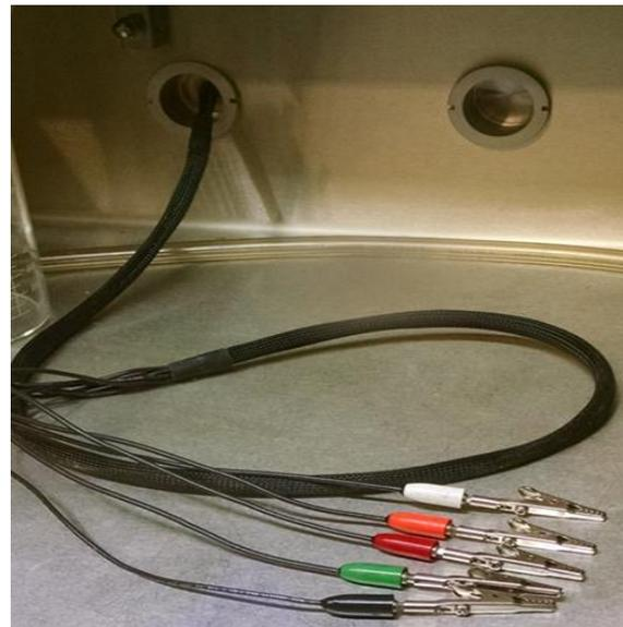
**Figure 3-2. Cell Cable Glovebox Feedthrough**
