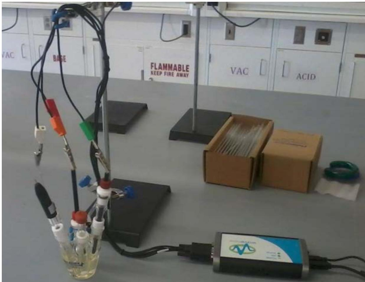
Figure 7. Electrochemical Cell (AKCELL1).
