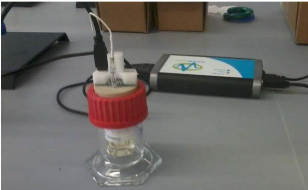
Figure 8. Mini Electrochemical Cell Setup
